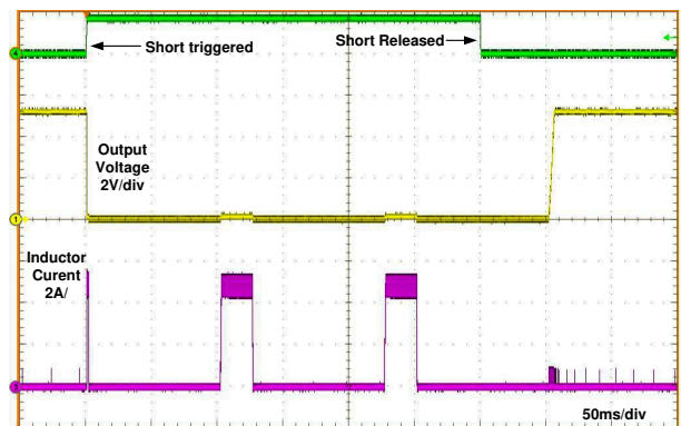
図 7-6. Short-Circuit Transient and Recovery
