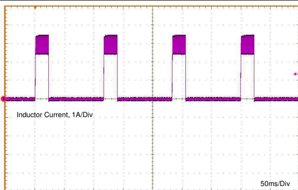
図 8-5. Inductor Current Burst in Short-Circuit Mode
