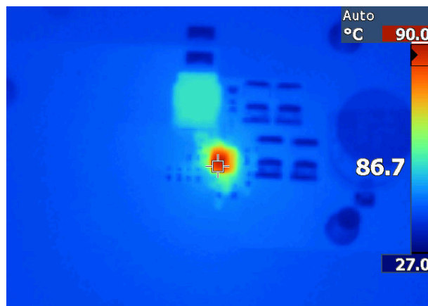
LMQ66430MC3 V_{OUT} = 3.3\text{ V} 12 V_{IN} , 3 A, 2.2 MHz Fixed
