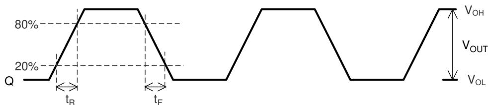
图 6. Output Voltage, and Rise and Fall Times
