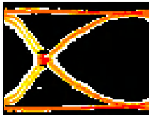
图 8-3. Internal Eye Monitor Hit Density Plot
