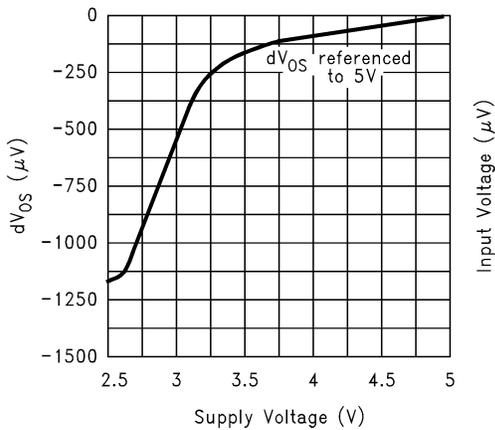
Figure 5-5.  $dV_{OS}$  vs Supply Voltage
