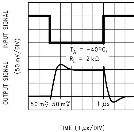
5-39. Inverting Small-Signal Pulse Response
