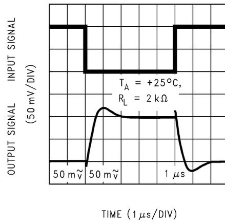
5-40. Inverting Small-Signal Pulse Response
