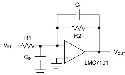
**Figure 7-2. Canceling the Effect of Input Capacitance**
