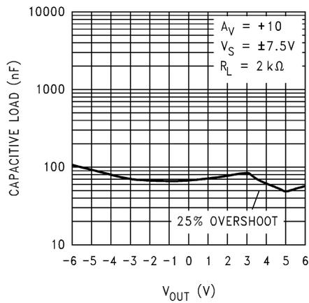
图 5-55. Stability vs Capacitive Load
