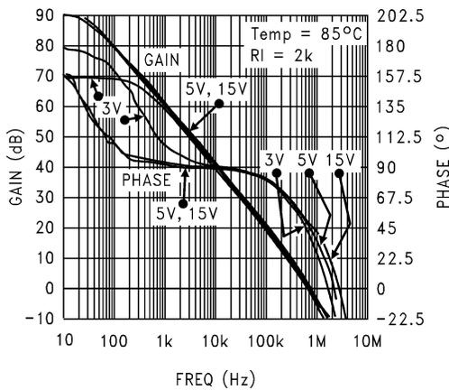
5-33. Open-Loop Frequency Response at  $85^\circ C$
