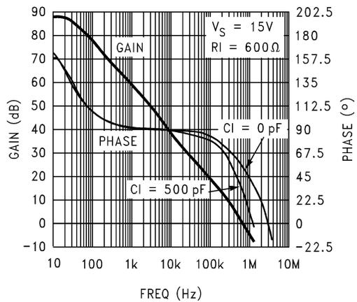
5-34. Gain and Phase vs Capacitive Load
