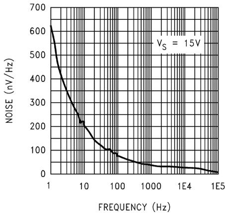
5-27. Input Voltage Noise vs Frequency
