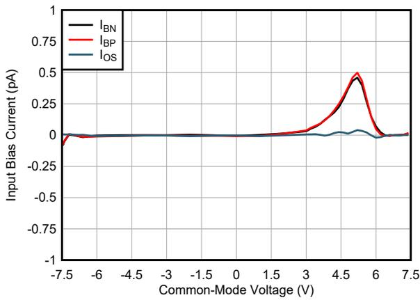
5-25. Input Bias Current vs Common-Mode Voltage
