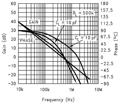
Figure 5-3. Gain and Phase vs Capacitance Load
