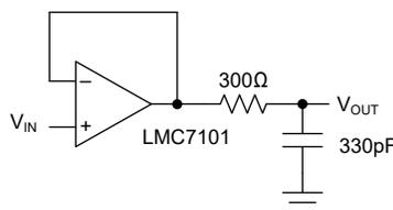
**図 7-1. Resistive Isolation of a 330pF Capacitive Load**
