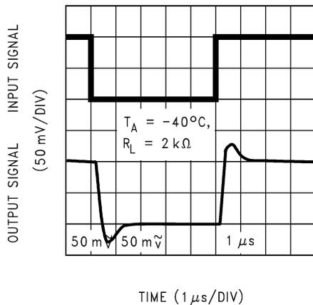
5-45. Noninverting Small-Signal Pulse Response
