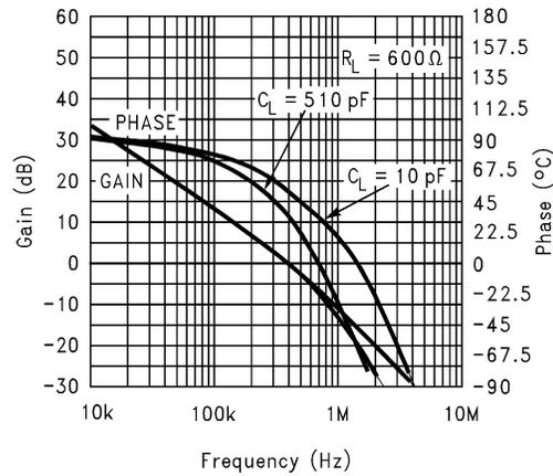
Figure 5-4. Gain and Phase vs Capacitance Load
