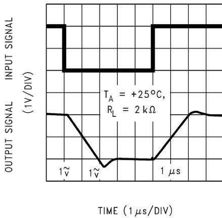
5-49. Noninverting Large-Signal Pulse Response
