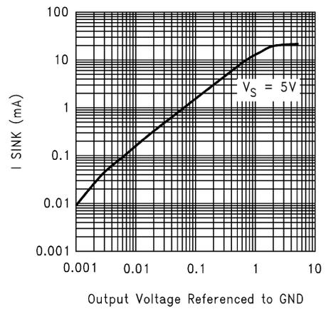
5-16. Sinking Current vs Output Voltage
