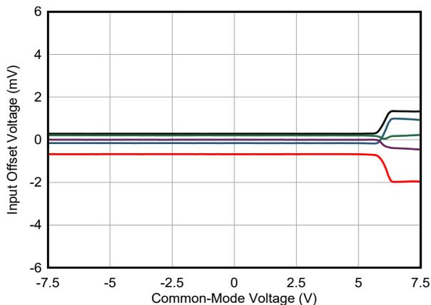
5-21. Input Offset Voltage vs Common-Mode Voltage
