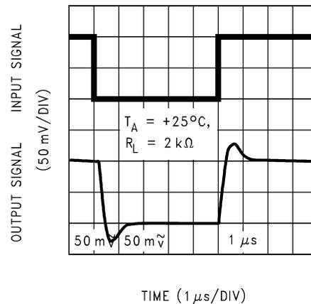
5-46. Noninverting Small-Signal Pulse Response
