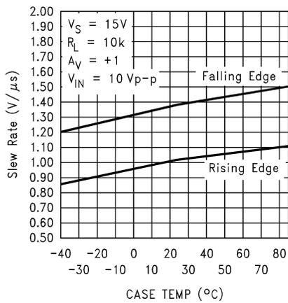
5-37. Slew Rate vs Temperature
