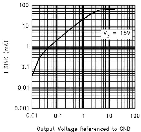
5-20. Sinking Current vs Output Voltage
