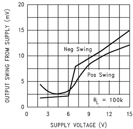
5-26. Output Voltage Swing vs Supply Voltage
