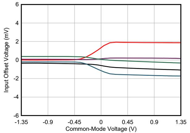
Figure 5-6. Input Offset Voltage vs Common-Mode Voltage
