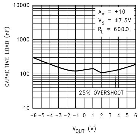
图 5-56. Stability vs Capacitive Load
