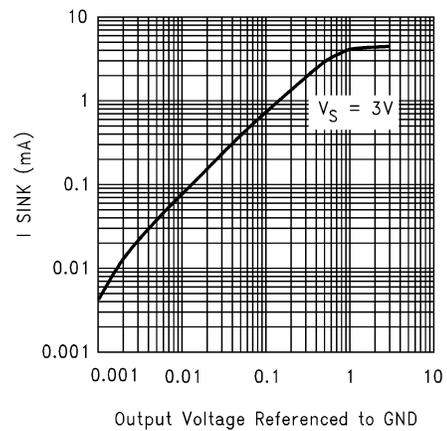
5-12. Sinking Current vs Output Voltage
