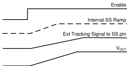
图 7-5. Tracking with Longer Start-up Time than the Internal Ramp
