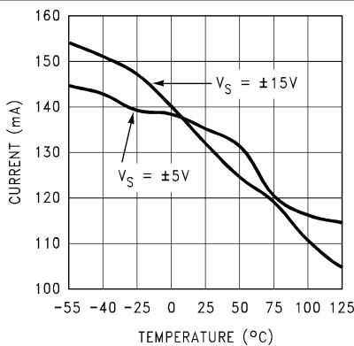
図 5-44. Short Circuit Current vs Temperature (Sourcing)
