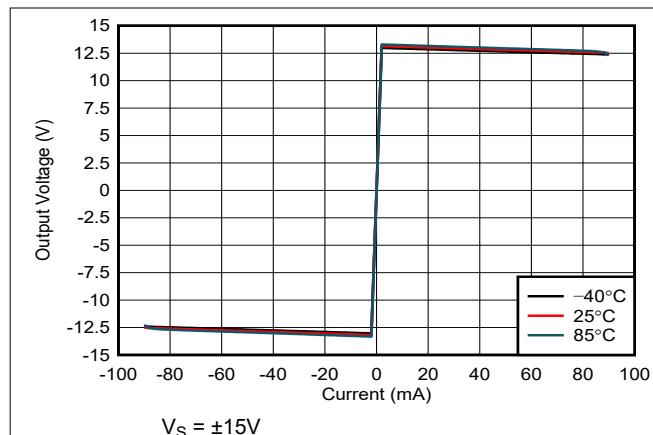
图 5-7. Output Voltage vs Output Current
