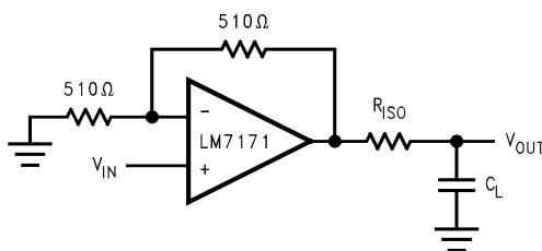
**図 6-9. Isolation Resistor Used to Drive Capacitive Load**
