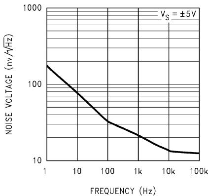
図 5-58. Input Voltage Noise vs Frequency
