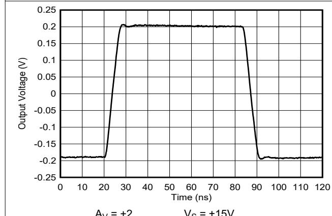
图 5-29. Small-Signal Pulse Response
