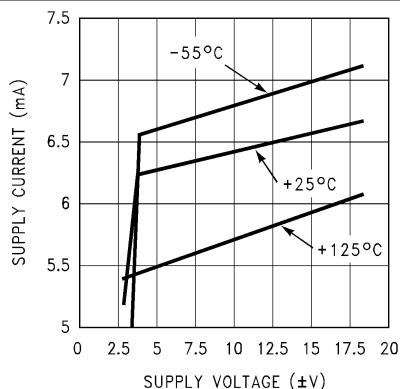
図 5-40. Supply Current vs Supply Voltage
