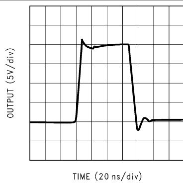
图 5-68. Large-Signal Pulse Response
