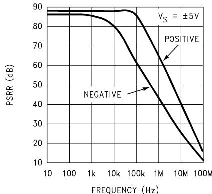
图 5-50. PSRR vs Frequency
