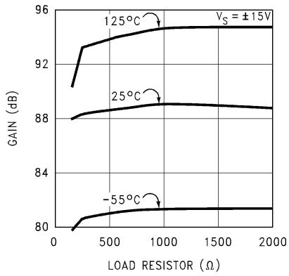
图 5-55. Large Signal Voltage Gain vs Load
