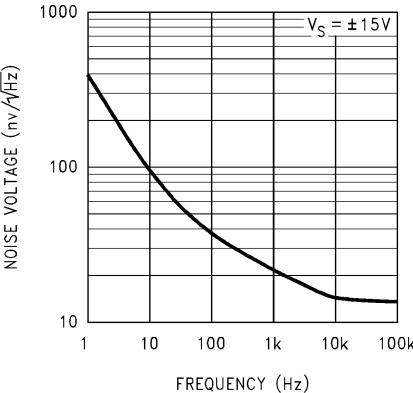
图 5-57. Input Voltage Noise vs Frequency
