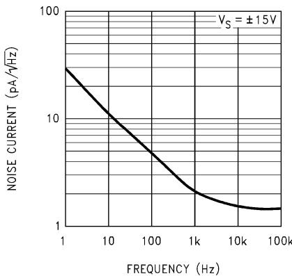
図 5-59. Input Current Noise vs Frequency
