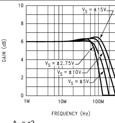
図 5-74. Closed-Loop Frequency Response vs Supply Voltage
