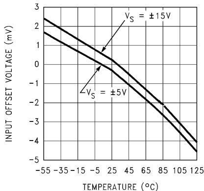
図 5-42. Input Offset Voltage vs Temperature
