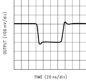
図 5-70. Small-Signal Pulse Response
