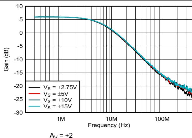
图 5-31. Closed-Loop Frequency Response vs Supply Voltage
