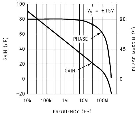
图 5-51. Open Loop Frequency Response
