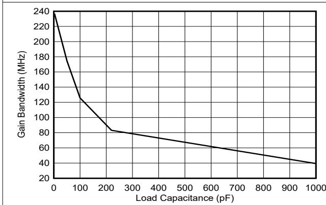
图 5-15. Gain-Bandwidth Product vs Load Capacitance
