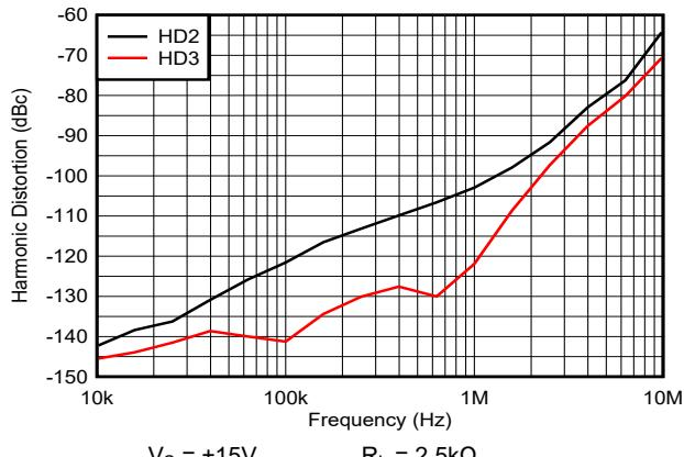
图 5-38. Harmonic Distortion vs Frequency
