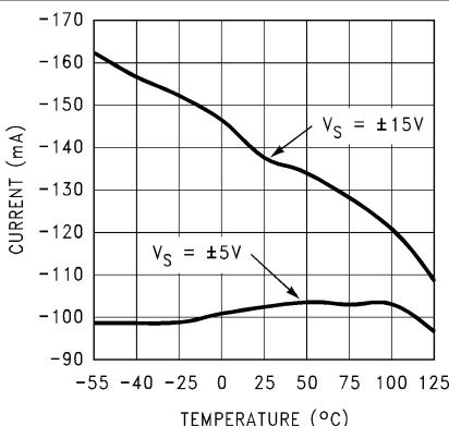
図 5-45. Short Circuit Current vs Temperature (Sinking)
