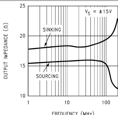
图 5-64. Open Loop Output Impedance vs Frequency
