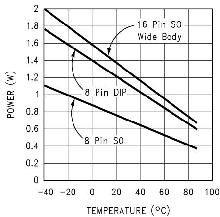
図 5-92. Maximum Power Dissipation vs Ambient Temperature
