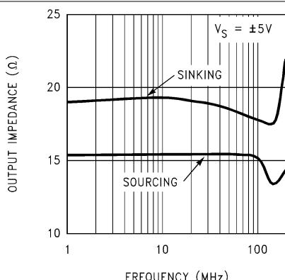
图 5-65. Open Loop Output Impedance vs Frequency
