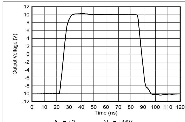
图 5-25. Large-Signal Pulse Response
