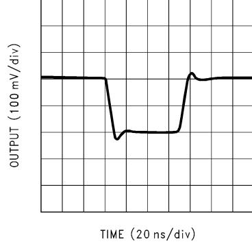
図 5-71. Small-Signal Pulse Response
