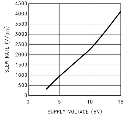
図 5-61. Slew Rate vs Supply Voltage
