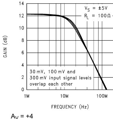
图 5-84. Closed-Loop Frequency Response vs Input Signal Level
