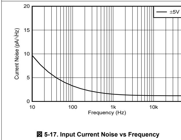
图 5-17. Input Current Noise vs Frequency
