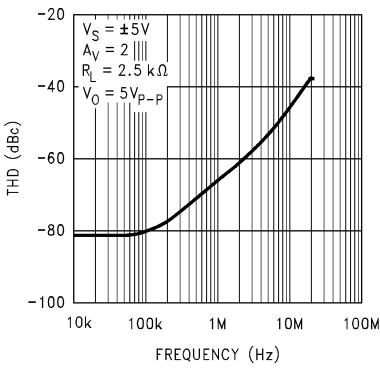
THD measurement at low frequency limited by test instrument
