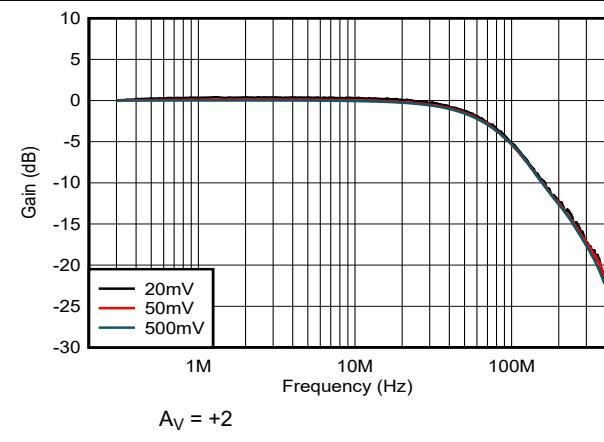
图 5-35. Closed-Loop Frequency Response vs Input Signal Level
