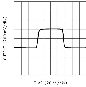
図 5-72. Small-Signal Pulse Response
