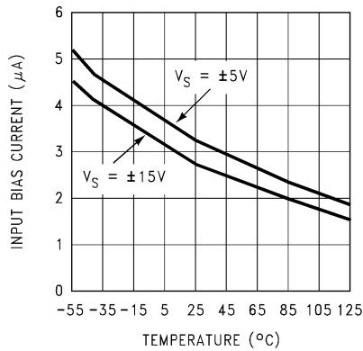
図 5-43. Input Bias Current vs Temperature
