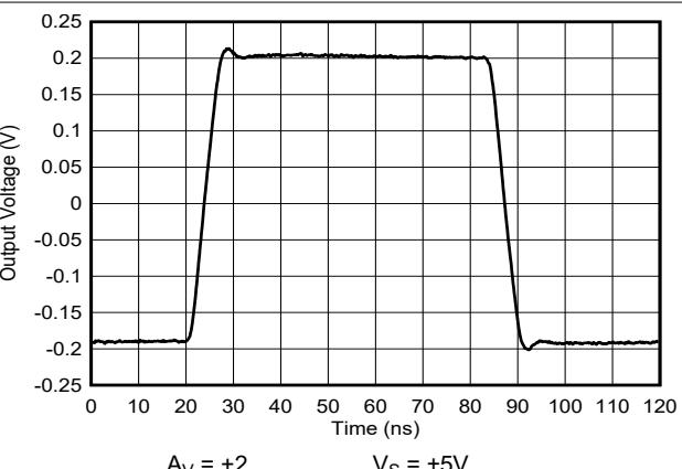
图 5-30. Small-Signal Pulse Response
