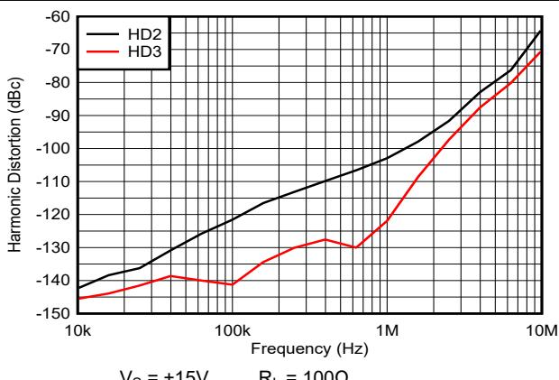
图 5-36. Total Harmonic Distortion vs Frequency
