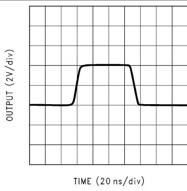
图 5-69. Large-Signal Pulse Response
