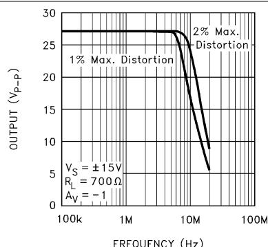
図 5-89. Undistorted Output Swing vs Frequency
