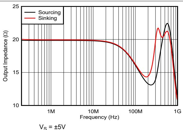
図 5-22. Open Loop Output Impedance vs Frequency
