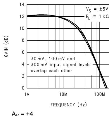
图 5-83. Closed-Loop Frequency Response vs Input Signal Level
