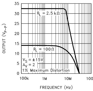
图 5-87. Undistorted Output Swing vs Frequency
