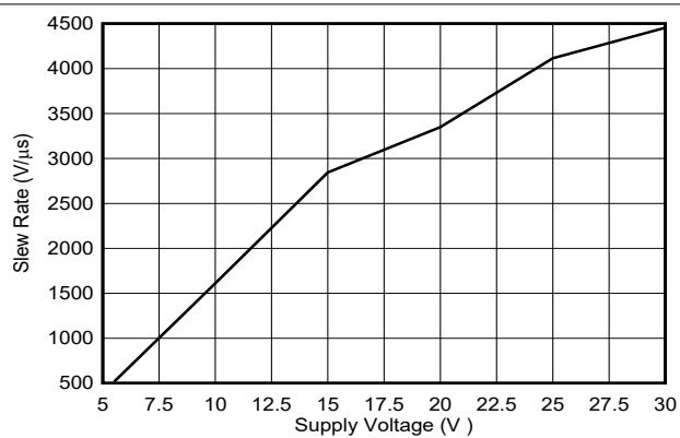
图 5-18. Slew Rate vs Supply Voltage
