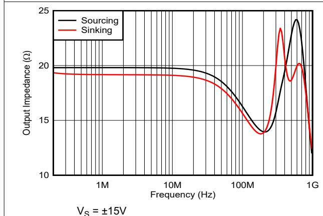
図 5-21. Open Loop Output Impedance vs Frequency
