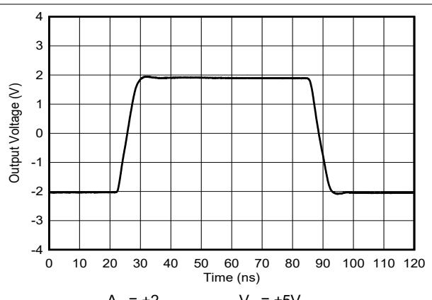
图 5-26. Large-Signal Pulse Response
