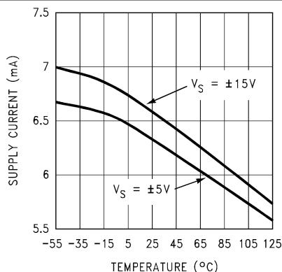
図 5-41. Supply Current vs Temperature
