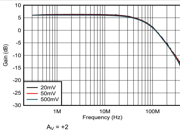
图 5-34. Closed-Loop Frequency Response vs Input Signal Level
