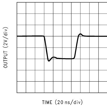
图 5-67. Large-Signal Pulse Response
