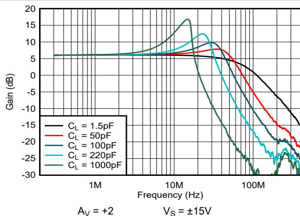
图 5-33. Closed-Loop Frequency Response vs Capacitive Load
