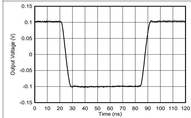
图 5-27. Small-Signal Pulse Response
