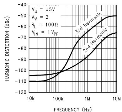
THD measurement at low frequency limited by test instrument
