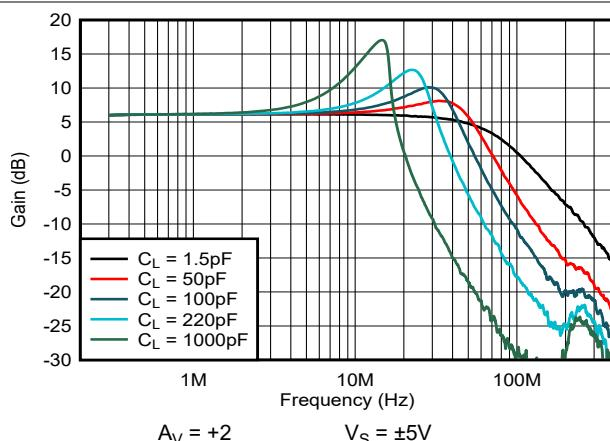
图 5-32. Closed-Loop Frequency Response vs Capacitive Load
