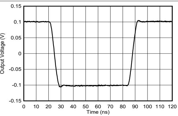
图 5-28. Small-Signal Pulse Response
