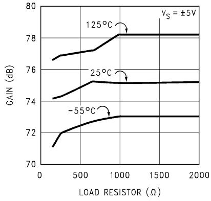
图 5-56. Large Signal Voltage Gain vs Load
