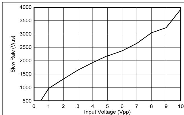
図 5-19. Slew Rate vs Input Voltage
