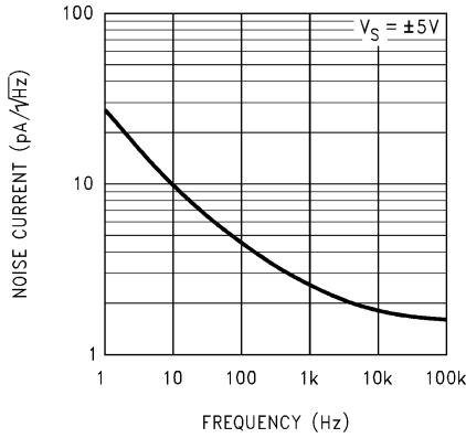
図 5-60. Input Current Noise vs Frequency
