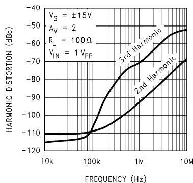
THD measurement at low frequency limited by test instrument
