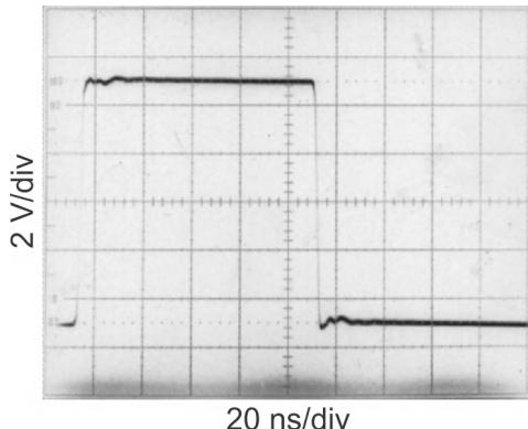
**図 6-7. Properly Terminated Signal**
