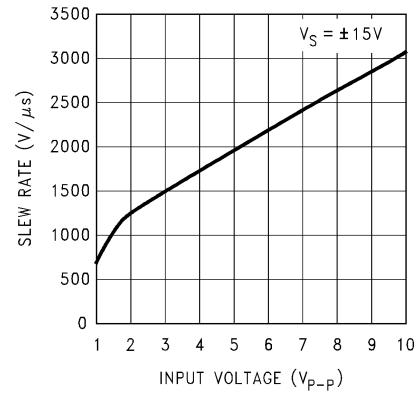
図 5-62. Slew Rate vs Input Voltage
