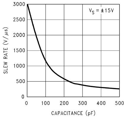
図 5-63. Slew Rate vs Load Capacitance
