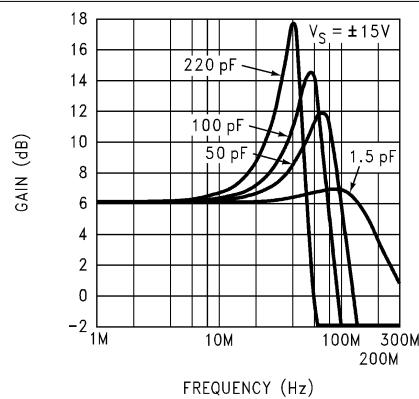
図 5-75. Closed-Loop Frequency Response vs Capacitive Load
