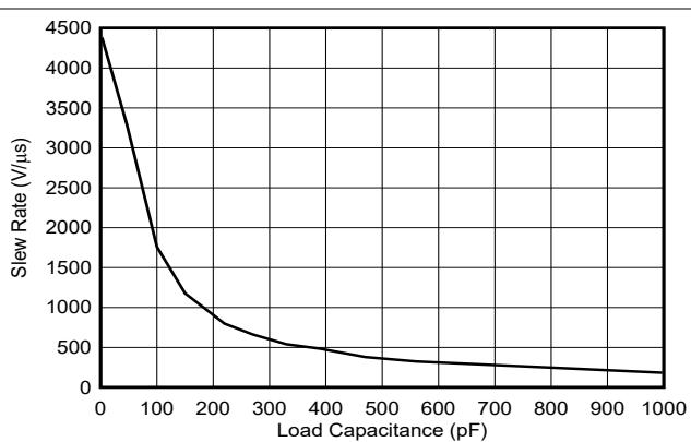
図 5-20. Slew Rate vs Load Capacitance
