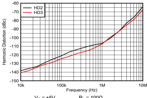
图 5-37. Total Harmonic Distortion vs Frequency
