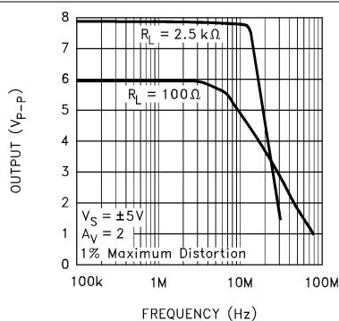
図 5-88. Undistorted Output Swing vs Frequency
