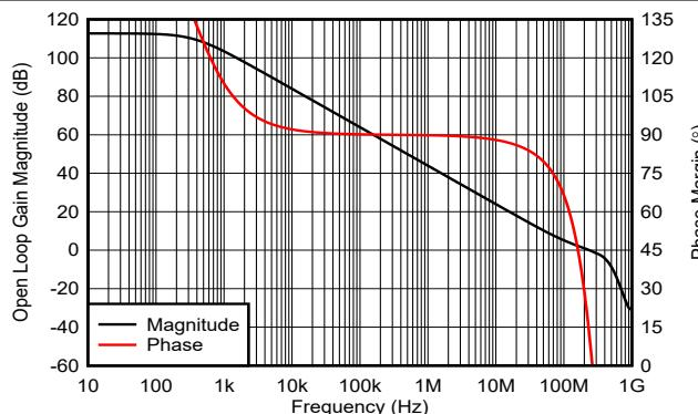
图 5-12. Open Loop Frequency Response
