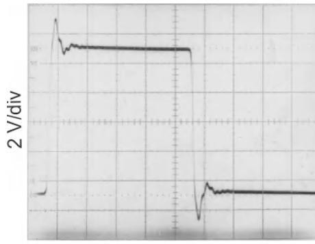
**図 6-8. Improperly Terminated Signal**
