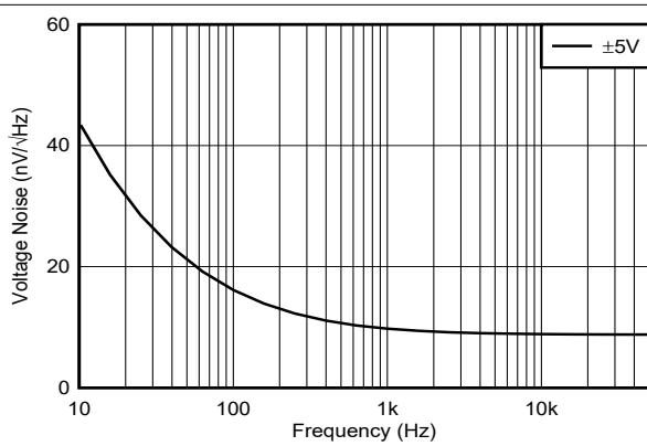
图 5-16. Input Voltage Noise vs Frequency
