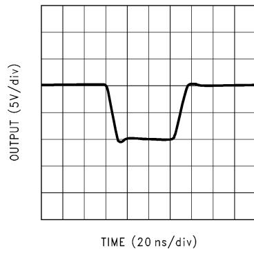
图 5-66. Large-Signal Pulse Response
