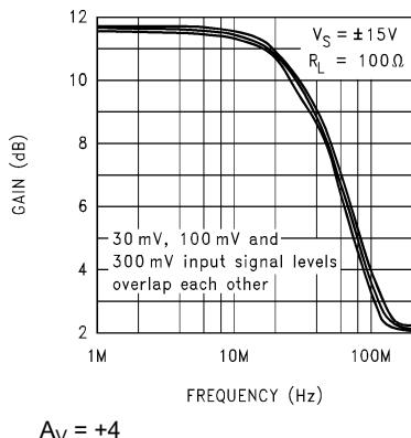
图 5-82. Closed-Loop Frequency Response vs Input Signal Level
