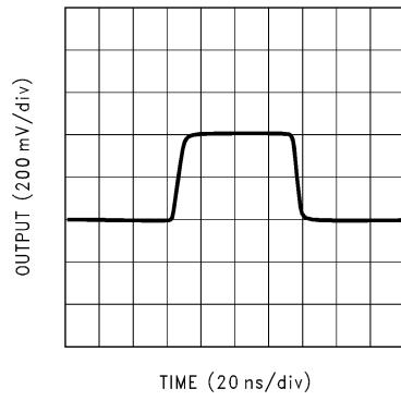
図 5-73. Small-Signal Pulse Response
