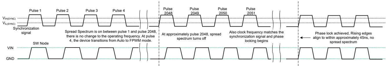
On the fourth pulse, the synchronization signal is detected. After approximately 2048 pulses, the synchronization signal is ready to synchronize, and the frequency is adjusted using a glitch-free technique, then the phase is locked.
