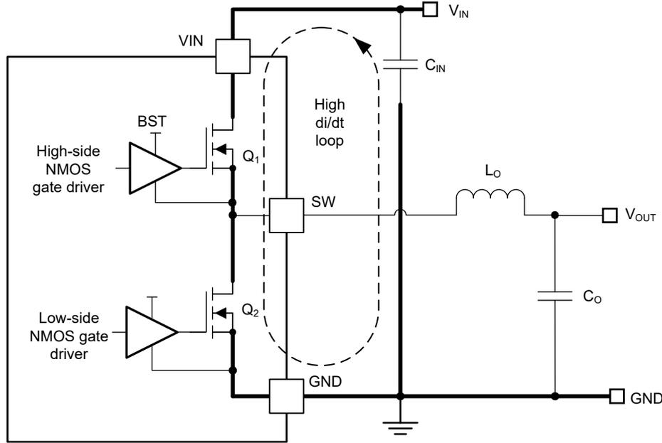
**図 8-5. Current Loops With Fast Edges**
