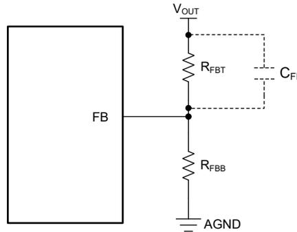
図 7-1. Setting Output Voltage of Adjustable Versions
