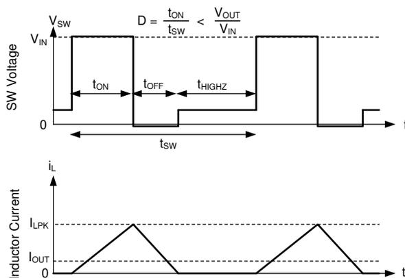
In auto mode, the low-side device is turned off after inductor current is near zero. As a result, after output current is less than half of inductor ripple in CCM, the part operates in DCM. This is equivalent to saying that diode emulation is active.
