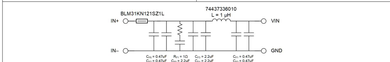
**Figure 8-55. Recommended Input EMI Filter**
