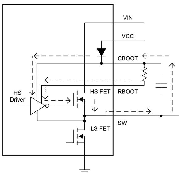
**Figure 7-10. Simplified Circuit Showing How RBOOT Functions**
