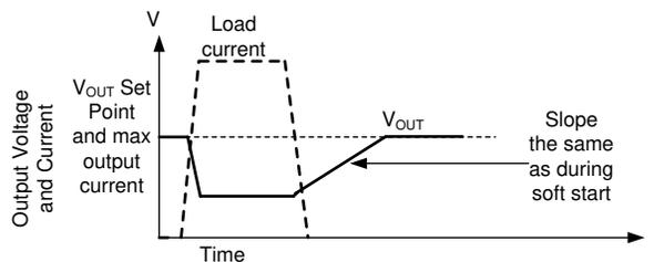
Whether output voltage falls due to high load or low input voltage, after the condition that causes output to fall below the setpoint is removed, output climbs at the same speed as during start-up. Even though hiccup does not trigger due to dropout, hiccup can, in principal, be triggered during recovery if output voltage is below 0.4 times the output setpoint for more than 128 clock cycles during recovery.
