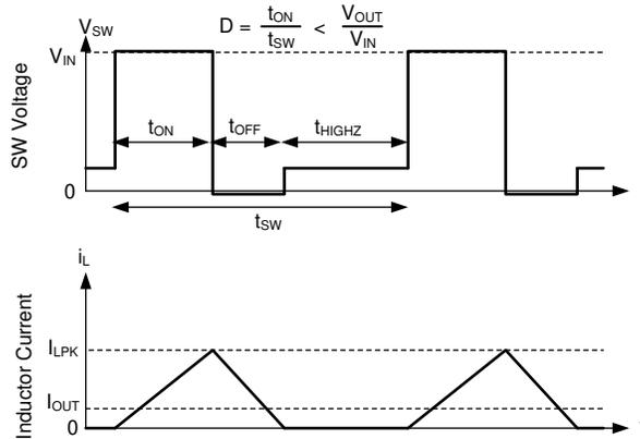
In auto mode, the low-side device is turned off after inductor current is near zero. As a result, after output current is less than half of inductor ripple in CCM, the part operates in DCM. This statement is equivalent to saying that diode emulation is active.
