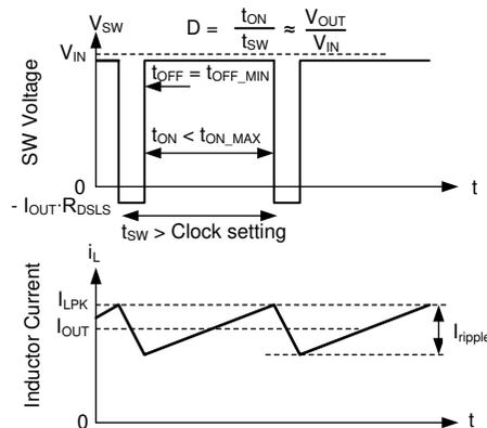
This image shows the switching waveforms while in dropout. Inductor current takes longer than a normal clock to reach the desired peak value. As a result, frequency drops. This frequency drop is limited by  $t_{ON\_MAX}$ .
