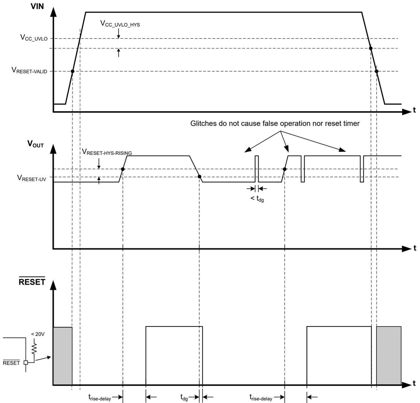
図 7-8. RESET Timing Diagram (Excludes OV Events)
