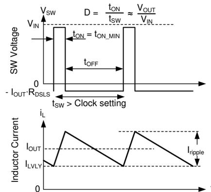
In valley control mode, the minimum inductor current is regulated, not peak inductor current.
