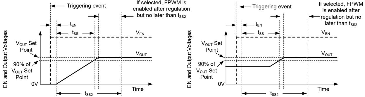
The left curves show soft start from 0V. The right curves show soft starting behavior from a prebiased or non-zero voltage. In either case, the output voltage reaches within 10% of the desired setpoint  $t_{SS}$  time after soft start is initiated. During soft start, FPWM and hiccup are disabled. Both hiccup and FPWM are enabled after output reaches regulation or  $t_{SS2}$ , whichever happens first.
