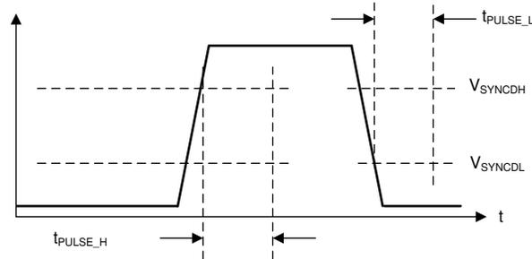
This image shows the conditions needed for detection of a synchronization signal.
