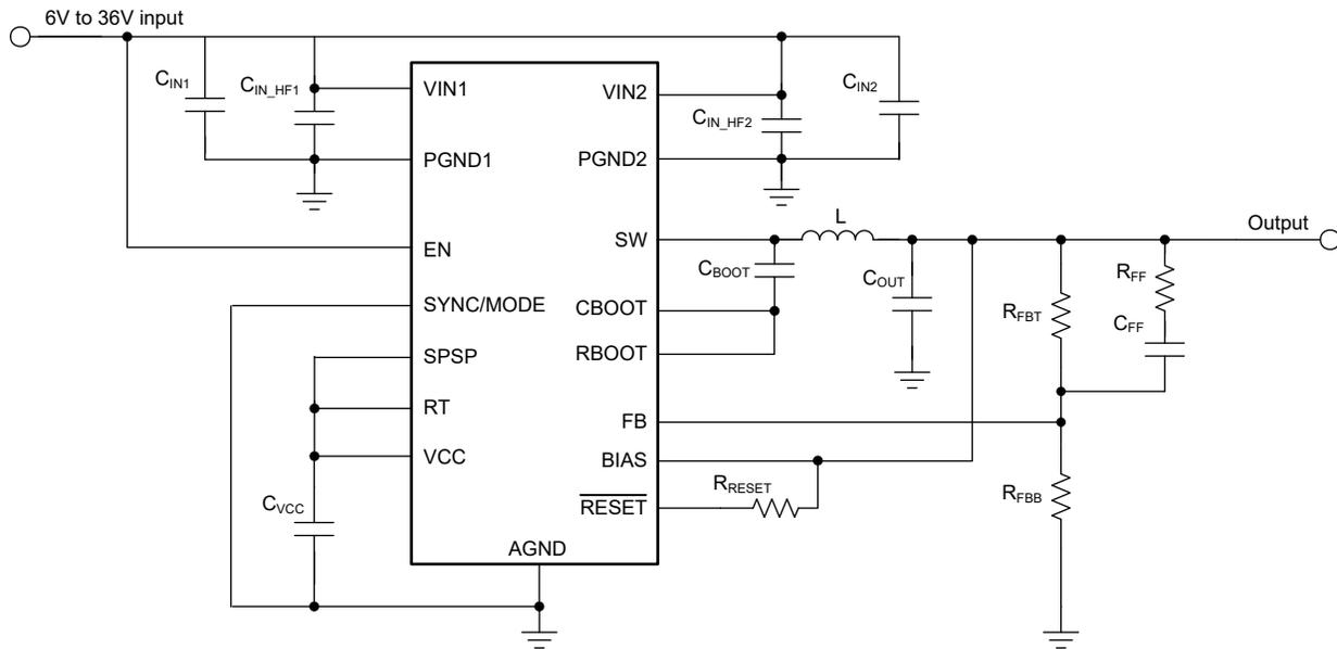
図 8-1. Example Application Circuit - 2.2MHz Adjustable Output
