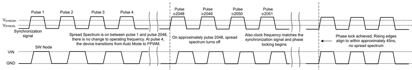
At pulse 4, the synchronization signal is detected. After approximately pulse 2048, the synchronization signal is ready to synchronize and the frequency is adjusted using a glitch-free technique. Later, phase is locked.
