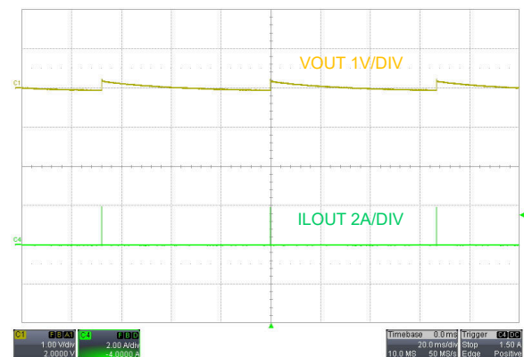
7-10. No Load Operation in PFM Mode, V_{SUPPLY} = 48V , I_{LOAD} = 0A
