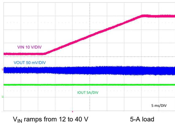
**9-34. Line Transient Response to  $V_{IN} = 40\text{ V}$**
