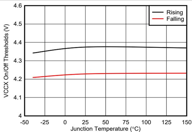
7-17. VCCX On and Off Thresholds vs Temperature
