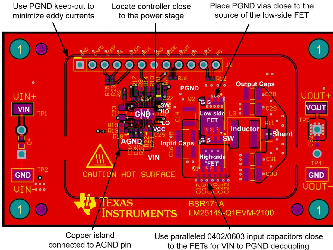
Figure 9-48. PCB Top Layer – High Density, Single-sided Design
