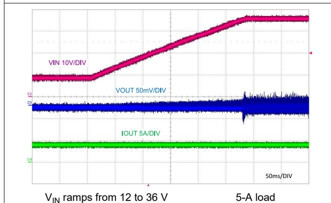
**9-10. Line Transient Response to V<sub>IN</sub> = 36 V**
