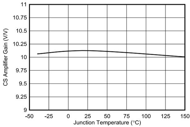
Figure 7-19. Current Sense (CS) Amplifier Gain vs Temperature
