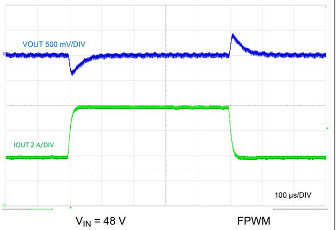
**图 9-28. Load Transient, 4 A to 8 A**
