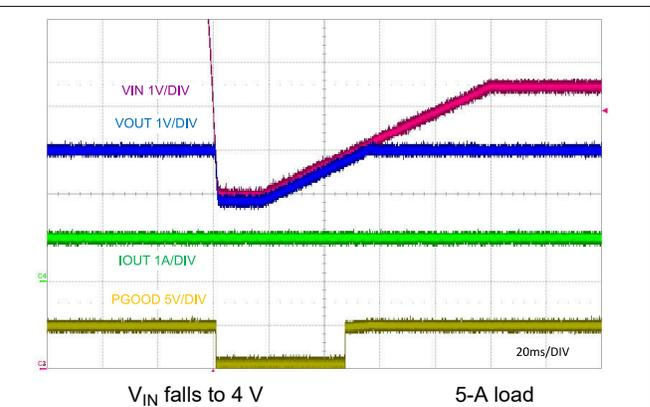
**9-11. Cold-Crank Response to V<sub>IN</sub> = 4 V**
