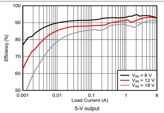
**9-7. Efficiency vs I<sub>OUT</sub>, Log Scale**
