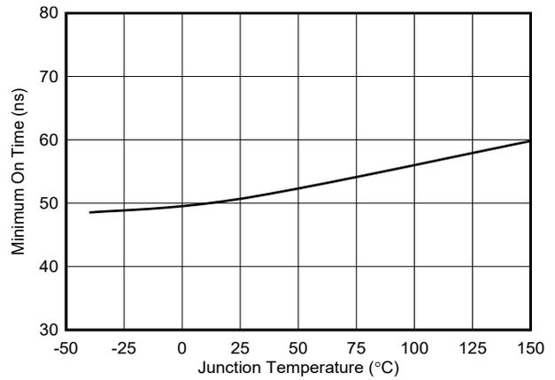
Figure 7-20. Minimum On Time (HO) vs Temperature
