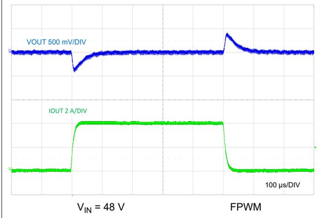
**图 9-27. Load Transient, 0 A to 4 A**
