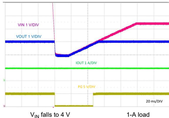
**9-35. Cold-Crank Response to  $V_{IN} = 4\text{ V}$**
