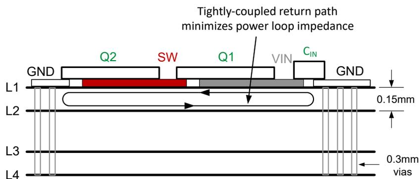
☒ 9-50. PCB Stack-up Diagram With Low L1-L2 Intra-layer Spacing <sup>1</sup>
