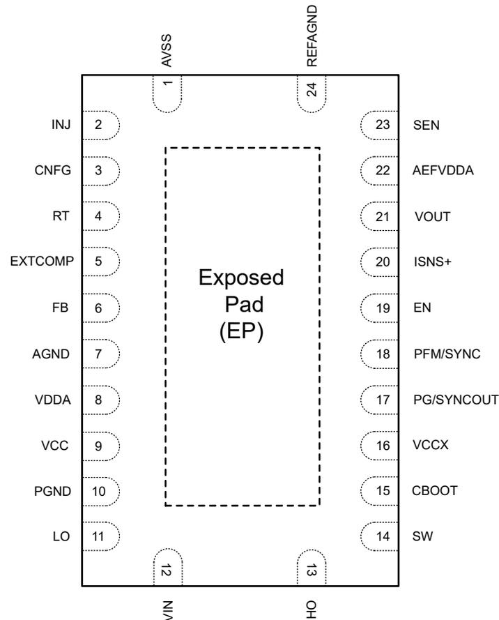
Connect the exposed pad to AGND and PGND on the PCB.
