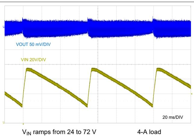
**9-24. Line Transient Response to  $V_{IN} = 72 V$**
