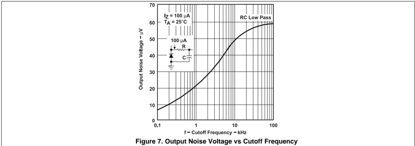
Figure 7. Output Noise Voltage vs Cutoff Frequency
