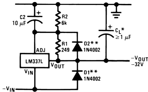
When  $C_L$  is larger than  $20 \mu\text{F}$ , D1 protects the LM337L in case the input supply is shorted.
