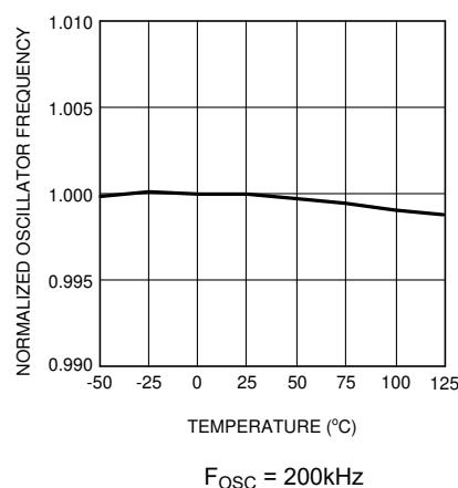
図 5-2. Oscillator Frequency vs Temperature
