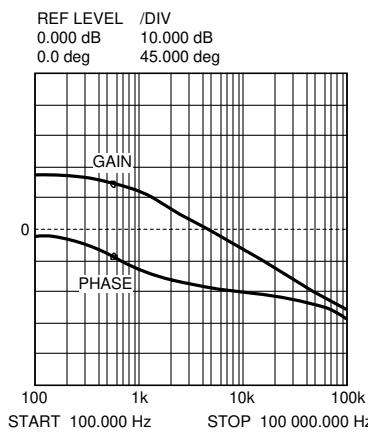
**図 7-3. Gain and Phase of Modulator  $R_{\text{LOAD}} = 20$  Ohms and  $C_{\text{OUT}} = 22\mu\text{F}$**
