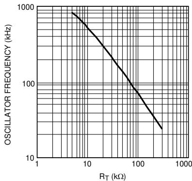
図 5-1. Oscillator Frequency vs  $R_T$
