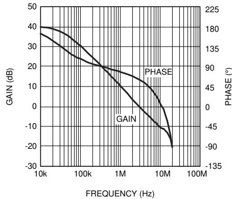
図 5-6. Error Amplifier Gain and Phase
