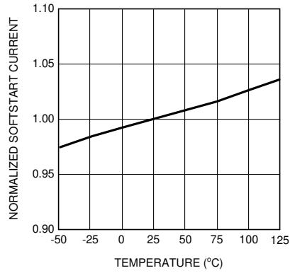
図 5-3. Soft Start Current vs Temperature
