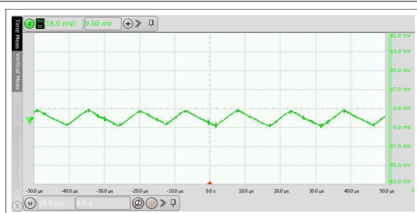
Figure 7-27. V_{ISOOUT} Ripple Voltage at 5 V with 10 \mu\text{F} Capacitor and 110 mA load
