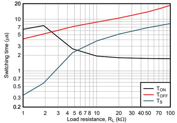
$I_F = 1.6mA$  ISOM8110 & ISOM8115  $V_{CC} = 5V$
