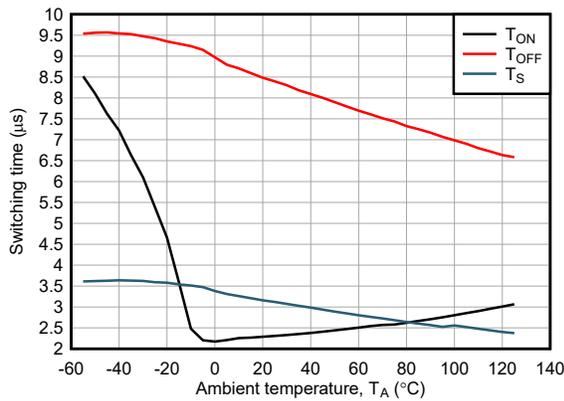
$I_F = 1.6\text{mA}$  ISOM8111 & ISOM8116  $V_{CC} = 5\text{V}$
