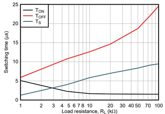
$I_F = 1.6mA$  ISOM8112 & ISOM8117  $V_{CC} = 5V$
