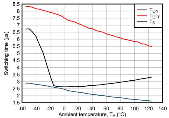
$I_F = 1.6\text{mA}$  ISOM8110 & ISOM8115  $V_{CC} = 5\text{V}$
