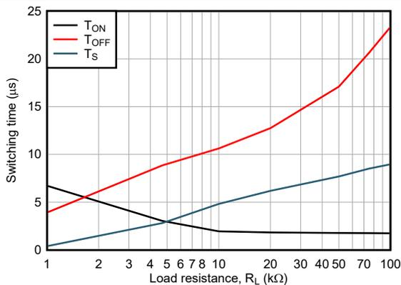
$I_F = 1.6mA$  ISOM8111 & ISOM8116  $V_{CC} = 5V$
