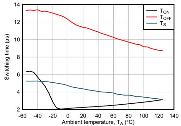
$I_F = 1.6\text{mA}$  ISOM8112 & ISOM8117  $V_{CC} = 5\text{V}$
