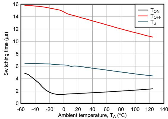
$I_F = 1.6\text{mA}$  ISOM8113 & ISOM8118  $V_{CC} = 5\text{V}$
