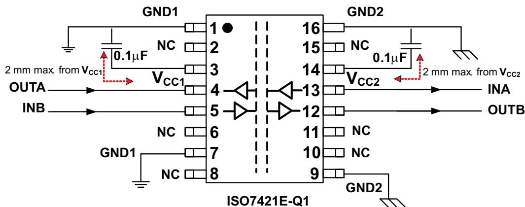
図 5. Typical ISO7421E-Q1 Application Circuit
