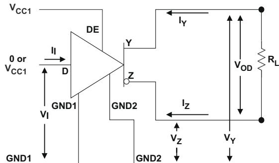
图 7-1. Driver  $V_{OD}$  Test and Current Definitions
