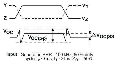
Input Generator PRR = 100 kHz, 50 % duty cycle,  $t_r < 6\text{ ns}$ ,  $t_f < 6\text{ ns}$ ,  $Z_O = 50\Omega$
