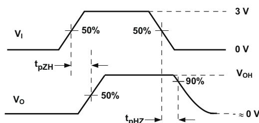
图 7-5. Driver High-Level Output Enable and Disable Time Test Circuit and Voltage Waveforms
