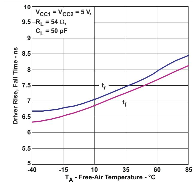
FIG 6-8. Driver Rise, Fall Time vs Free-Air Temperature
