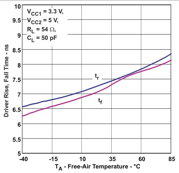
FIG 6-9. Driver Rise, Fall Time vs Free-Air Temperature
