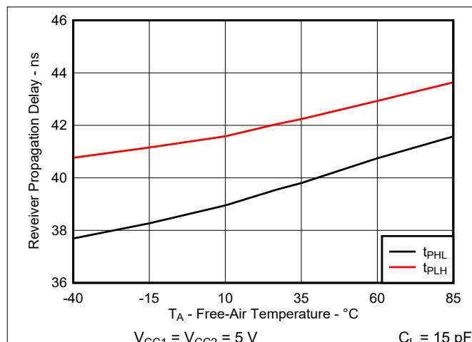
FIG 6-6. Receiver Propagation Delay vs Free-Air Temperature
