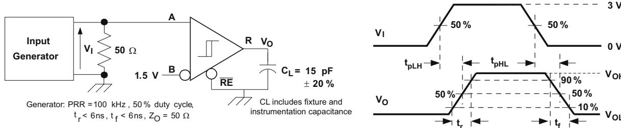
图 7-8. Receiver Switching Test Circuit and Waveforms
