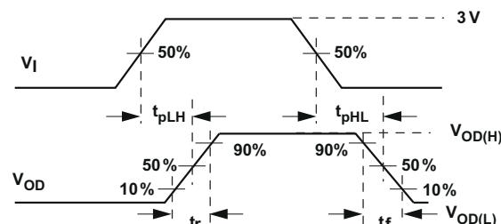
图 7-4. Driver Switching Test Circuit and Voltage Waveforms
