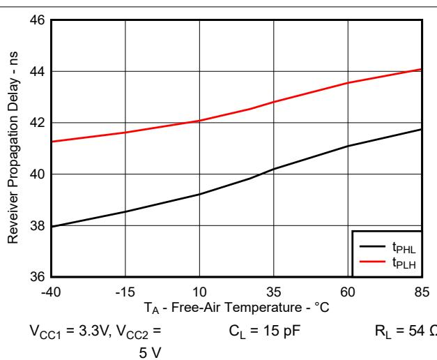
FIG 6-7. Receiver Propagation vs Free-Air Temperature
