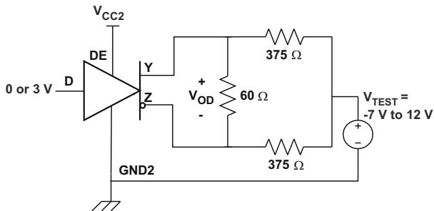
图 7-2. Driver  $V_{OD}$  With Common-Mode Loading Test Circuit
