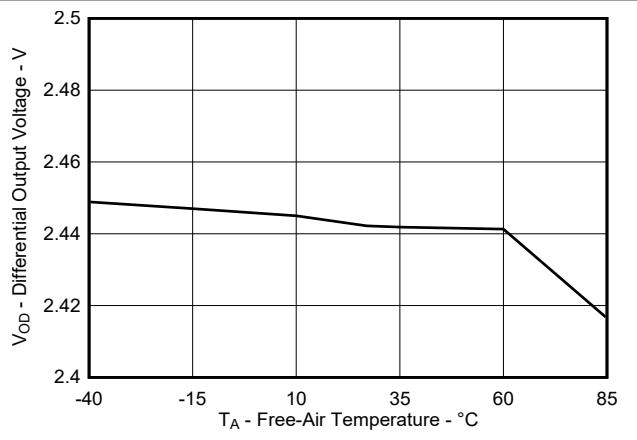
图 6-16. Differential Output Voltage vs Free-Air Temperature
