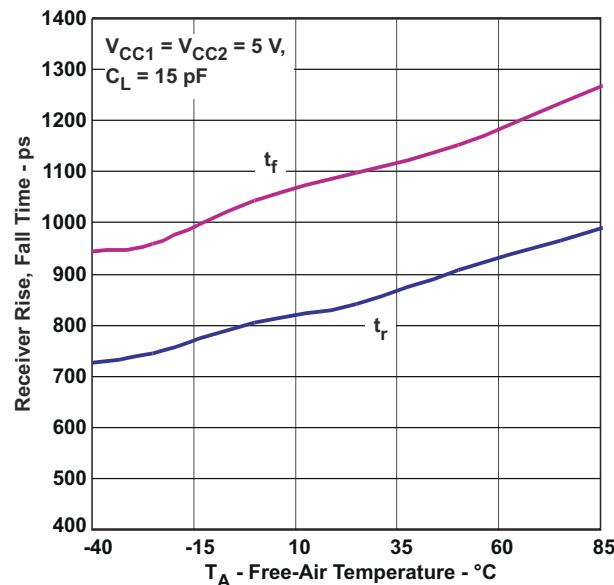
FIG 6-10. Receiver Rise, Fall Time vs Free-Air Temperature
