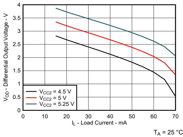
FIG 6-12. Driver Differential Output Voltage vs Load Current
