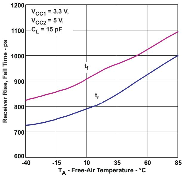
FIG 6-11. Receiver Rise, Fall Time vs Free-Air Temperature
