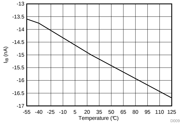
FIG 11. Input Bias Current vs Temperature
