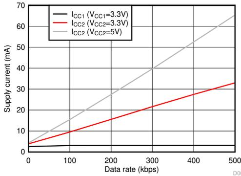
DE = V<sub>CC1</sub> RE = GND1 T<sub>A</sub> = 25°C
