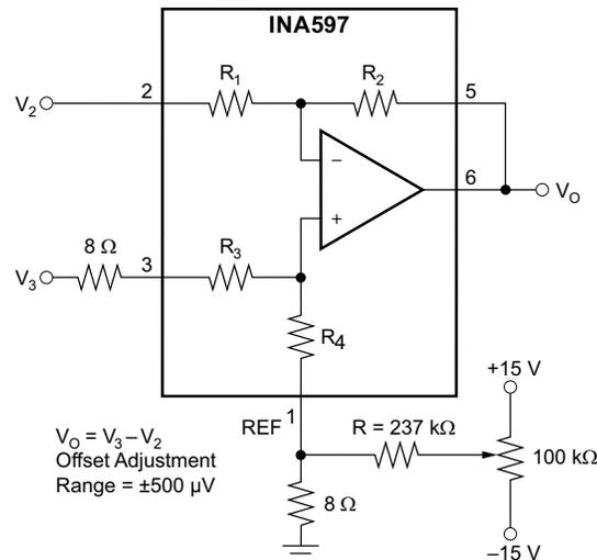
NOTE: For  $\pm 750\text{-}\mu\text{V}$  range,  $R = 158\text{ k}\Omega$ .
