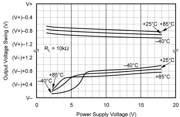
图 6-14. Output Voltage Swing vs Power Supply Voltage
