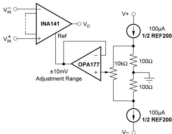
図 7-2. Optional Trimming of Output Offset Voltage.
