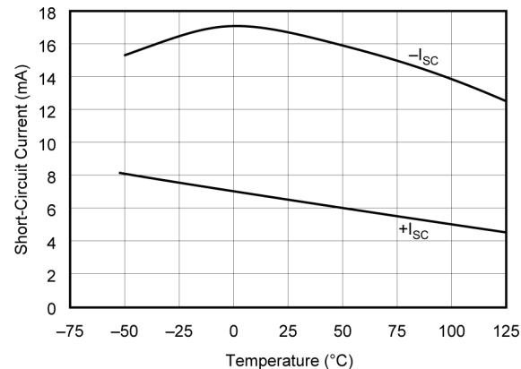
图 6-15. Short-circuit Output Current vs Temperature
