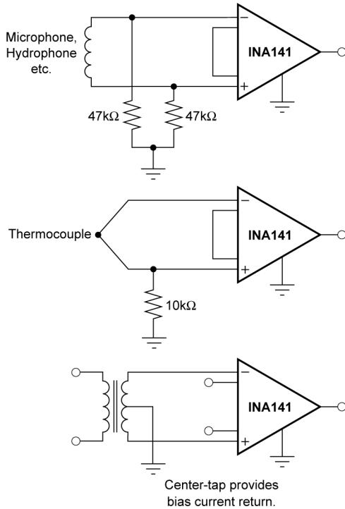
図 7-3. Providing an Input Common-Mode Current Path.
