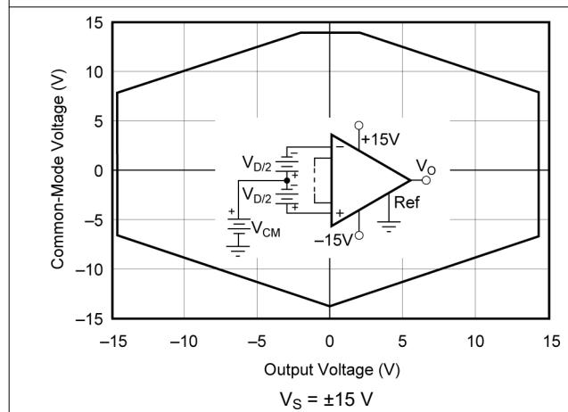
**图 6-5. Input Common-Mode Range vs Output Voltage**
