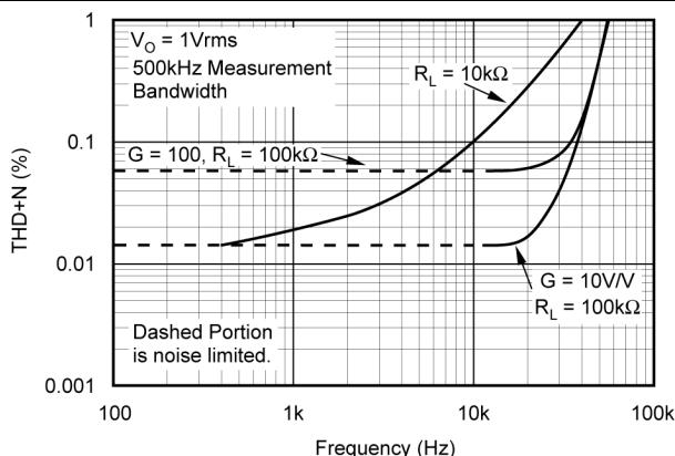
图 6-17. Total Harmonic Distortion + Noise vs Frequency
