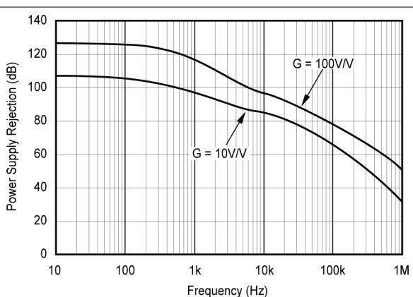
**图 6-4. Negative Power Supply Rejection vs Frequency**
