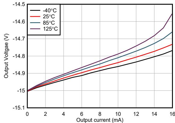
图 6-13. Negative Output Voltage Swing vs Output Current
