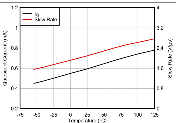
图 6-8. Quiescent Current and Slew Rate vs Temperature
