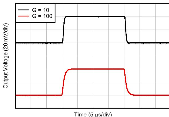
图 6-18. Small-Signal Step Response
