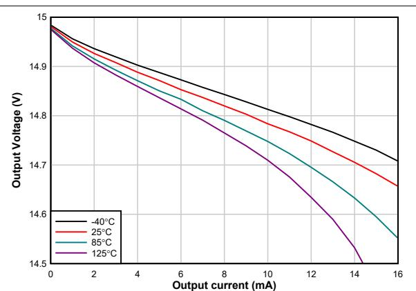
图 6-12. Positive Output Voltage Swing vs Output Current
