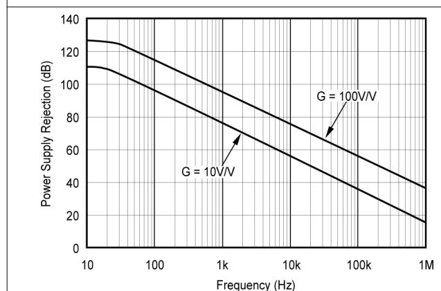
**图 6-3. Positive Power Supply Rejection vs Frequency**
