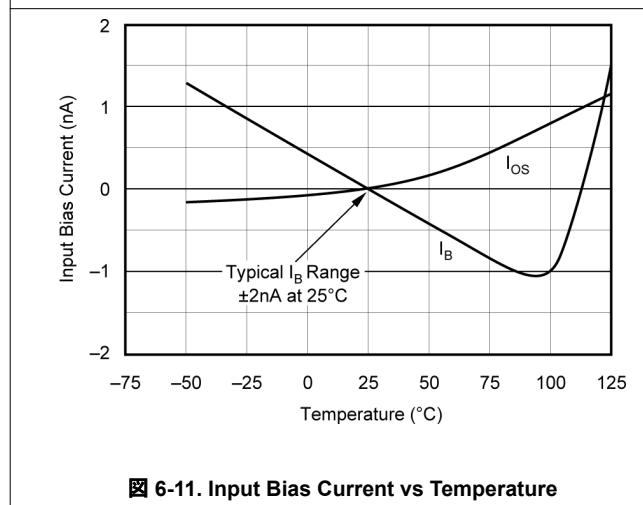
图 6-11. Input Bias Current vs Temperature
