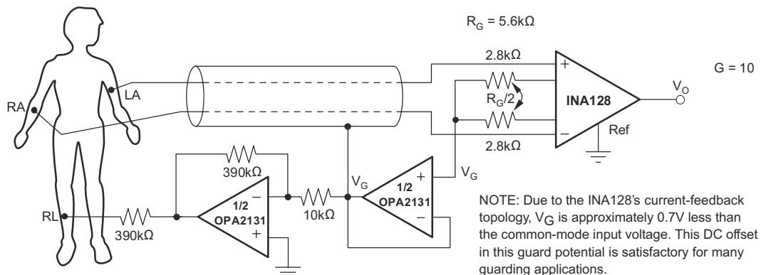
図 9-12. ECG Amplifier With Right-Leg Drive
