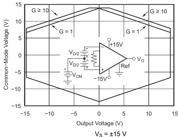
图 7-5. Input Common-Mode Range vs Output Voltage
