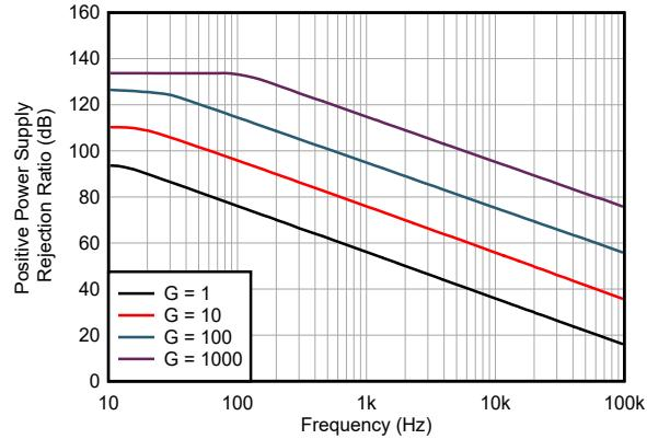
图 7-3. Positive Power Supply Rejection vs Frequency
