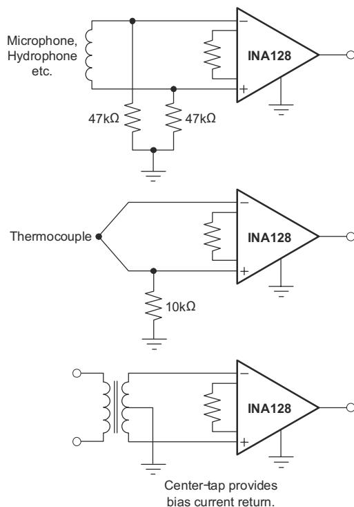
**图 9-3. Providing an Input Common-Mode Current Path**
