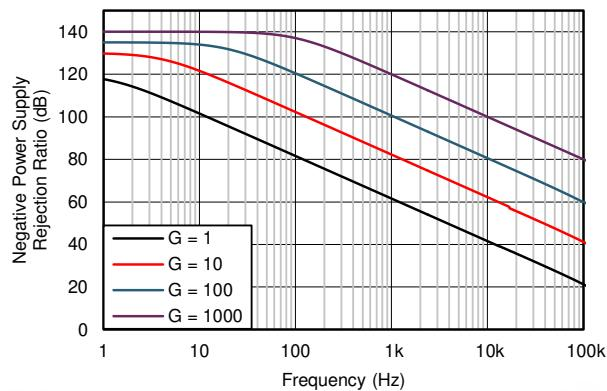
图 7-4. Negative Power Supply Rejection vs Frequency
