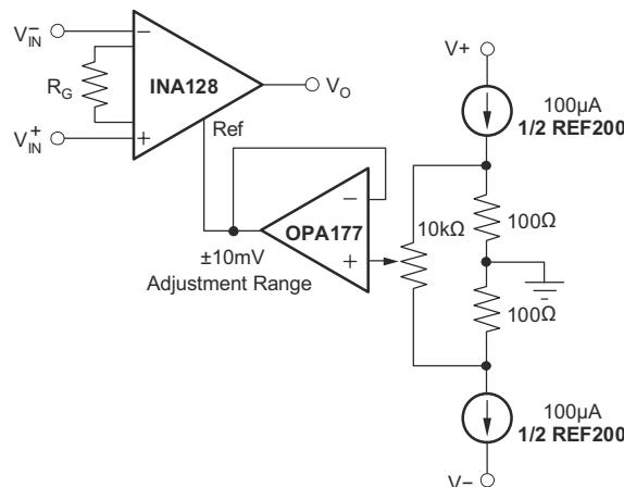
**图 9-2. Optional Trimming of Output Offset Voltage**
