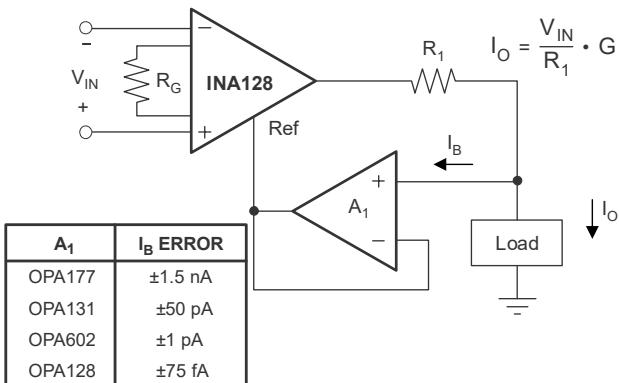
図 9-11. Differential Voltage to Current Converter
