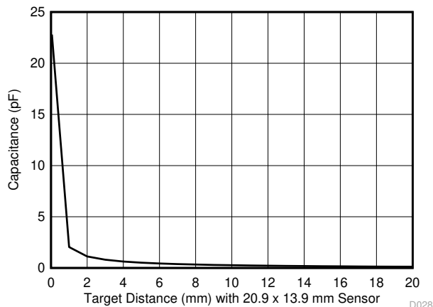
Figure 7-4. FDC2212 / FDC2214: Capacitance vs Target Distance (0mm to 20mm)
