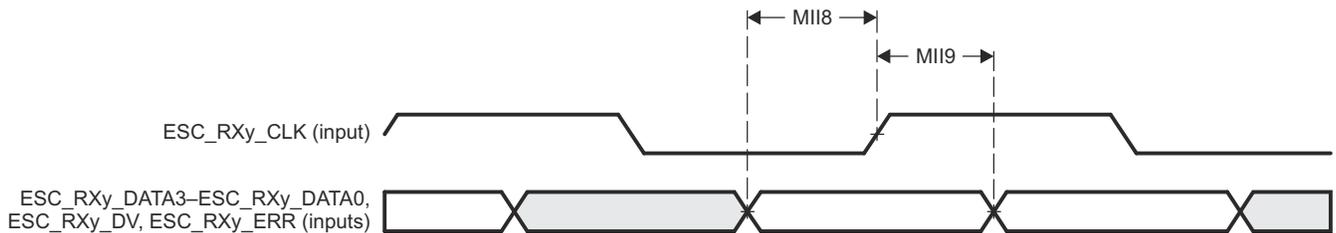
**Figure 6-87. EtherCAT Receive Interface Timing (MII Operation)**
