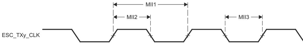
**Figure 6-84. EtherCAT Transmit Clock Timing (MII Operation)**
