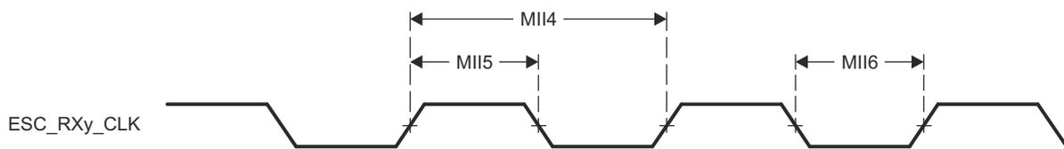
**Figure 6-86. EtherCAT Receive Clock Timing (MII Operation)**
