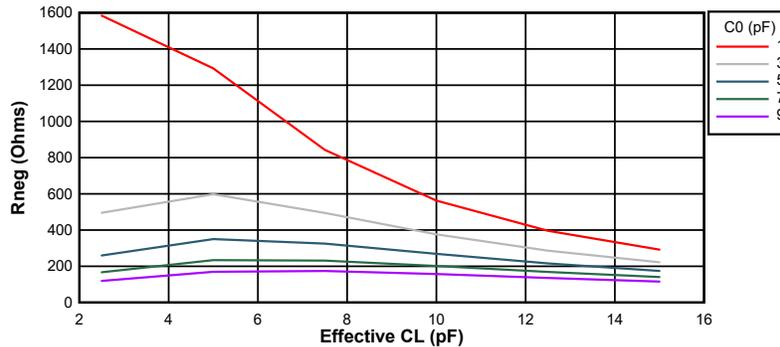
**Figure 6-15. Negative Resistance Variation at 20 MHz**
