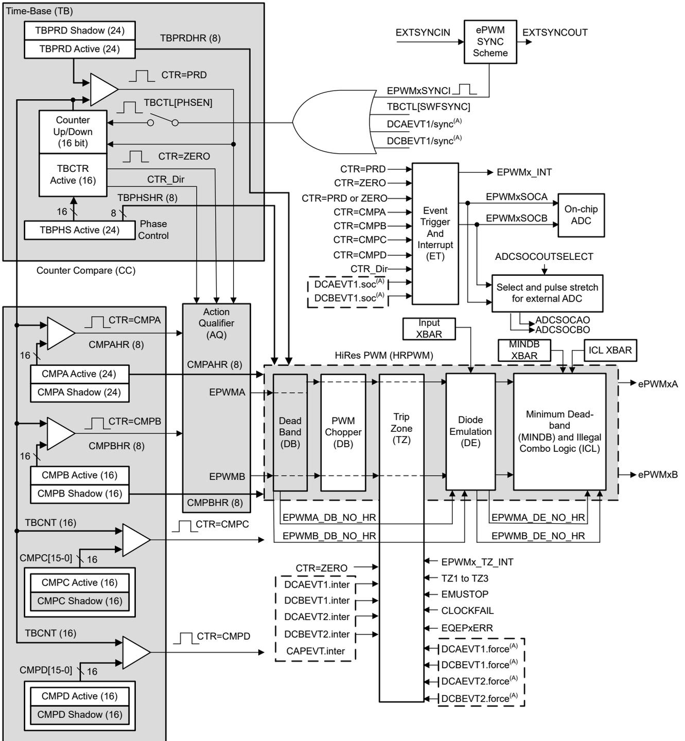
A. These events are generated by the ePWM digital compare (DC) submodule based on the levels of the TRIPIN inputs.
