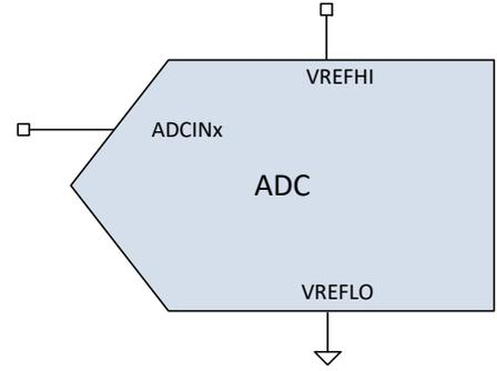
**Figure 6-37. Single-ended Signaling Mode**
