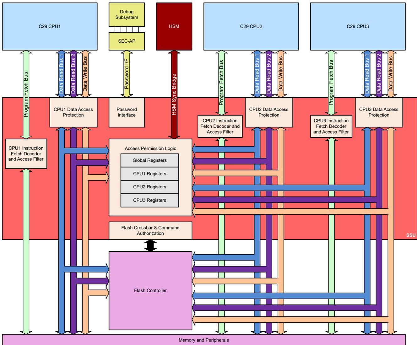
Figure 7-12. C29 Real-Time Security Architectural Block Diagram
