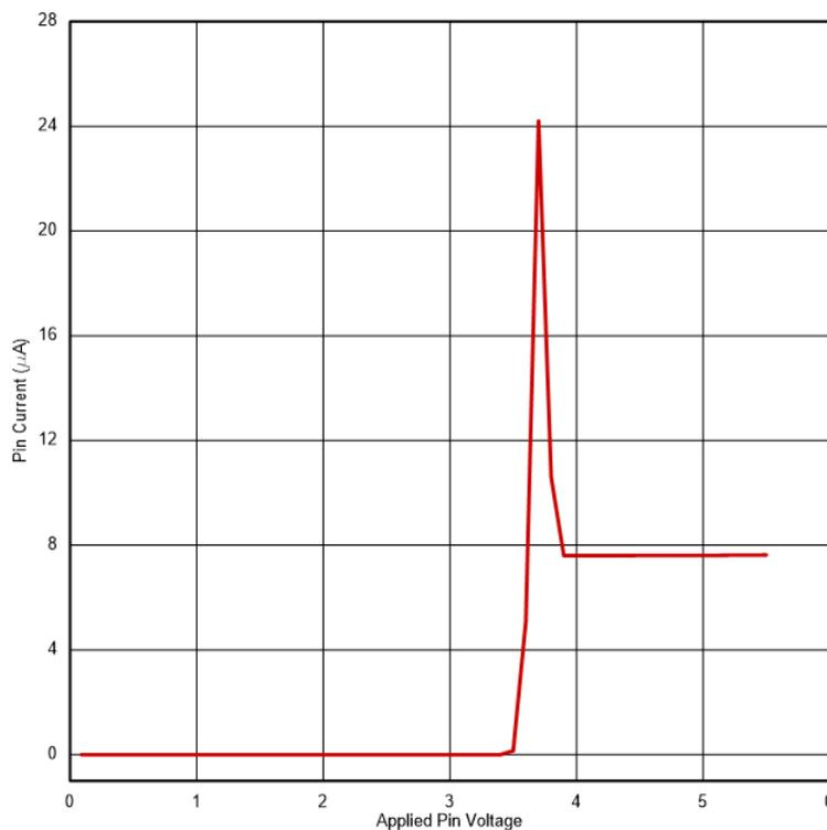
**Figure 6-1. Leakage Current vs Input Voltage (Device Powered)**
