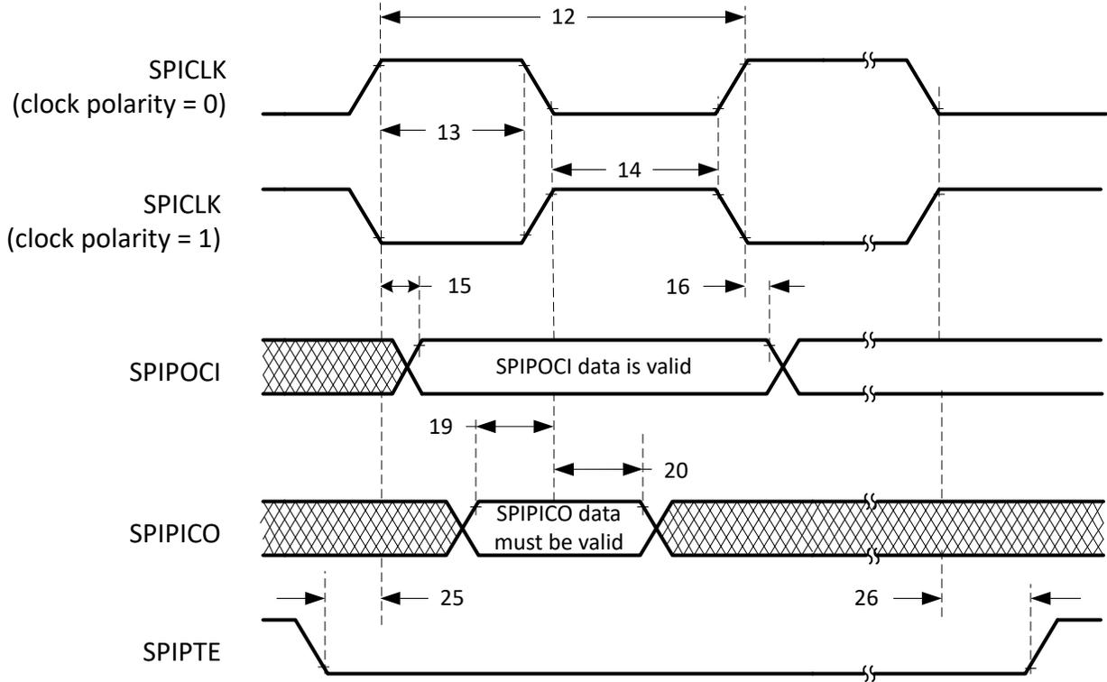
Figure 6-80. SPI Peripheral Mode External Timing (Clock Phase = 0)
