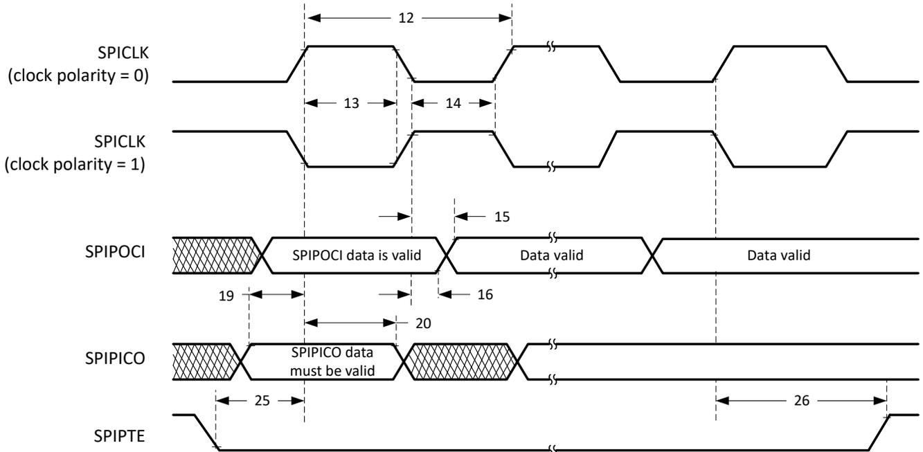
Figure 6-81. SPI Peripheral Mode External Timing (Clock Phase = 1)
