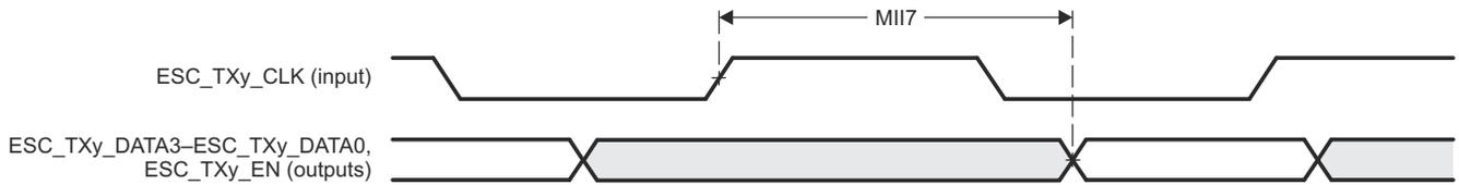
**Figure 6-85. EtherCAT Transmit Interface Timing (MII Operation)**
