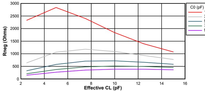
**Figure 6-14. Negative Resistance Variation at 10 MHz**
