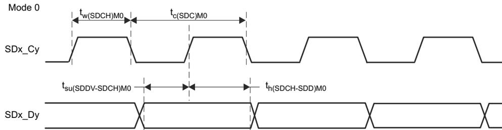
**Figure 6-65. SDFM Timing Diagram – Mode 0**
