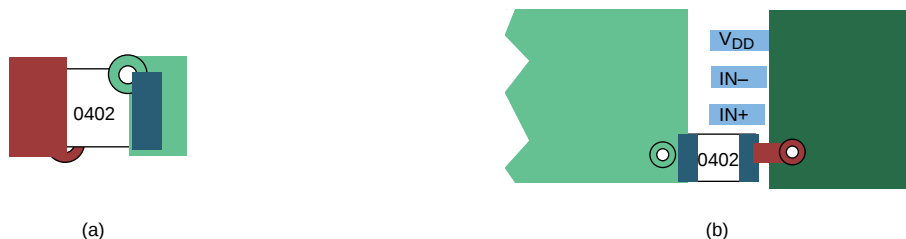
Figure 21. Typical Decoupling Capacitor Layouts
