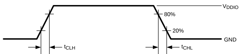
Figure 10. Deserializer LVCMOS Transition Times
