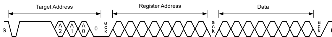
图 7-31. Serial Control Bus — WRITE
