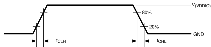
4-1. LVCMOS Transition Times
