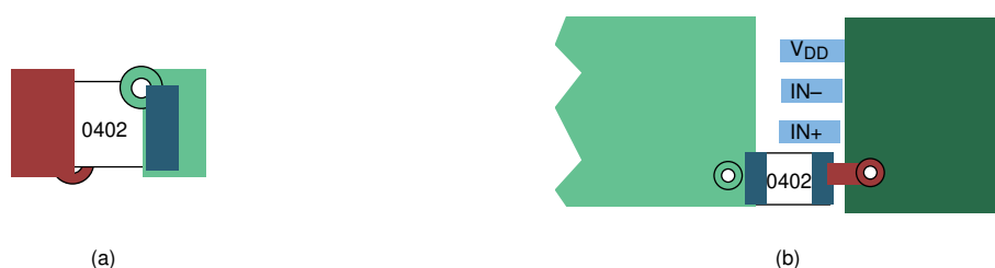
Figure 21. Typical Decoupling Capacitor Layouts
