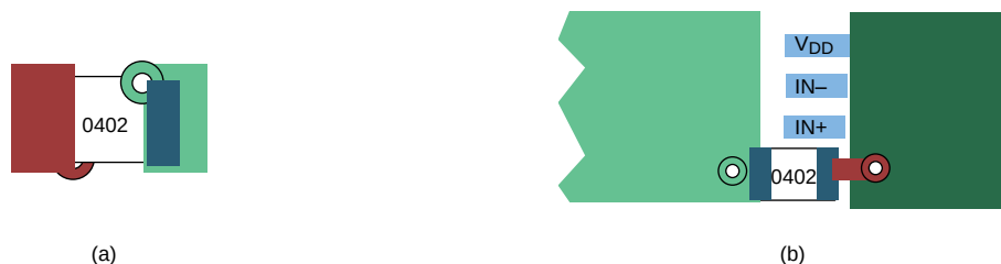
Figure 27. Typical Decoupling Capacitor Layouts
