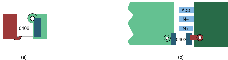
Figure 11-7. Typical Decoupling Capacitor Layouts
