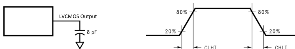
Figure 2. LVCMOS Output Load and Transition Times
