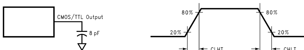
Figure 4. DS90CF3x6 (Receiver) CMOS or LVC MOS Output Load and Transition Times
