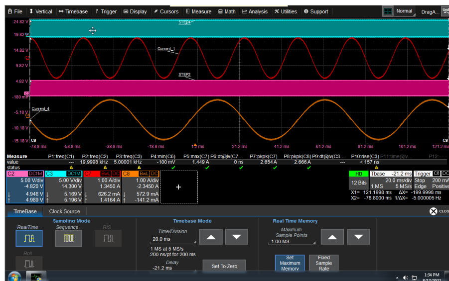
9-2. DRV8849 driving two Stepper Motors
