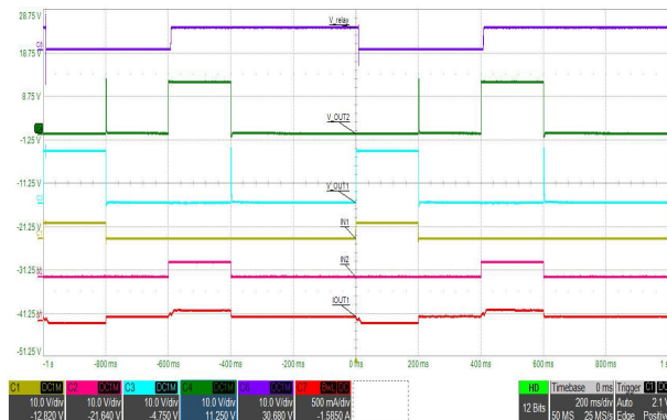
A. Ch 1 = IN1 Ch 2 = IN2 Ch 3 = V_{OUT1} Ch 4 = V_{OUT2} Ch 6 = Relay Switch Ch 7 = Relay Coil Current
