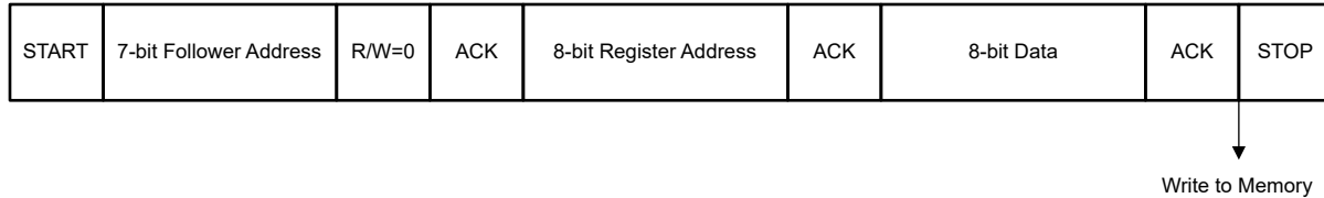
図 8-20. I 2 C Write Sequence
