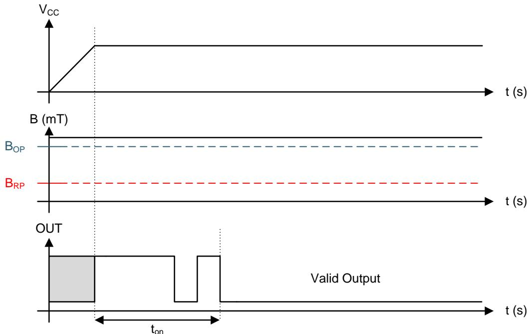
**Figure 13. Case 1: Power On When  $B > B_{OP}$**
