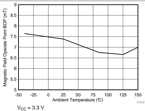
**Figure 4. DRV5033-Q1AJ,  $B_{OP}$  vs Temperature**
