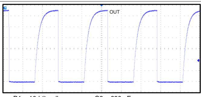
**Figure 20. 10-kHz Switching Magnetic Field**
