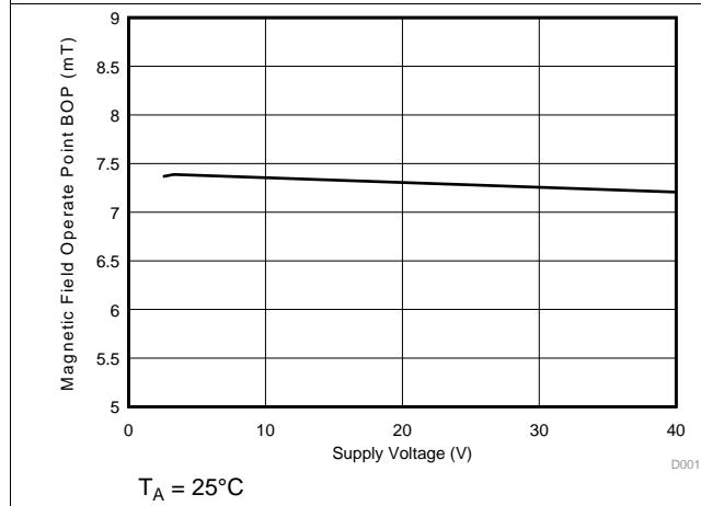
**Figure 3. DRV5033-Q1AJ,  $B_{OP}$  vs  $V_{CC}$**
