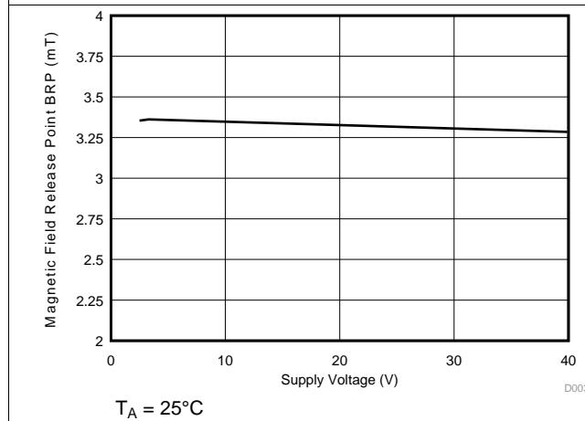
**Figure 5. DRV5033-Q1AJ,  $B_{RP}$  vs  $V_{CC}$**
