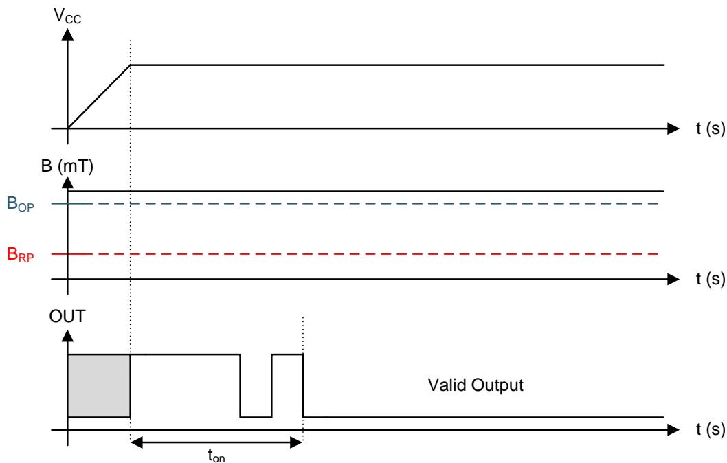
**Figure 14. Case 1: Power On When  $B > B_{OP}$**
