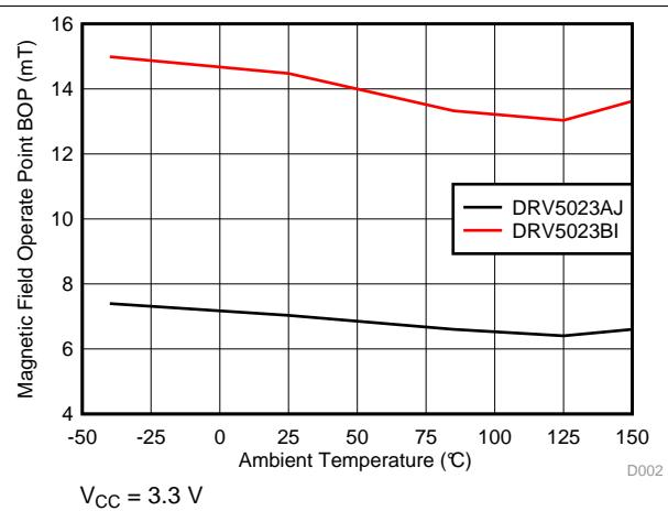
**Figure 4.  $B_{OP}$  vs Temperature**
