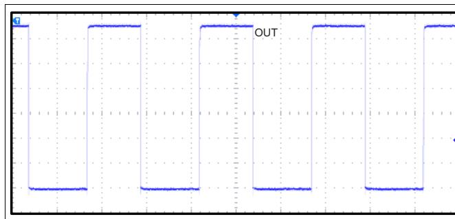
**Figure 21. 10-kHz Switching Magnetic Field**
