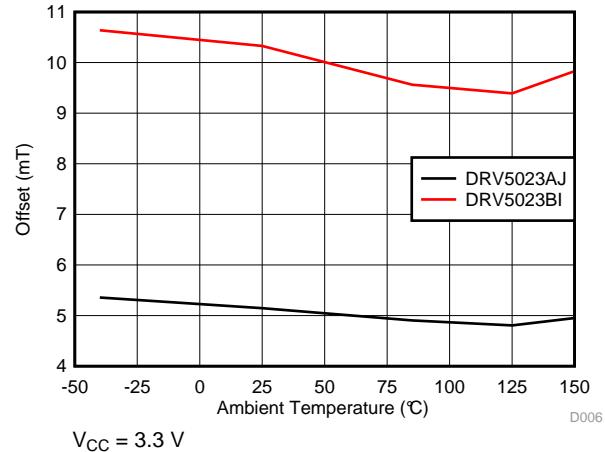
**Figure 10. Offset vs Temperature**
