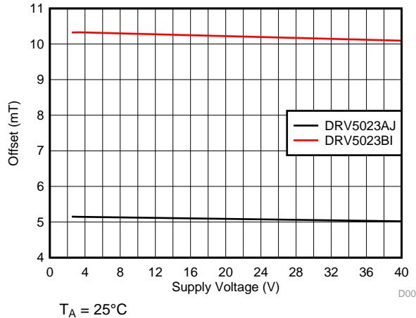
**Figure 9. Offset vs  $V_{CC}$**
