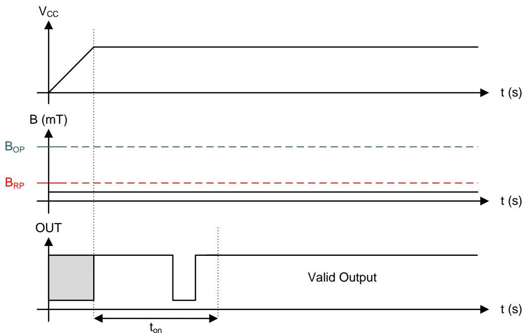
**Figure 15. Case 2: Power On When  $B < B_{RP}$**
