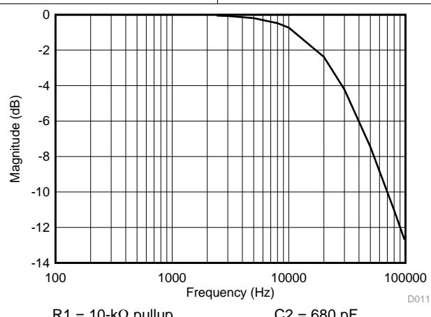
**Figure 23. Low-Pass Filtering**
