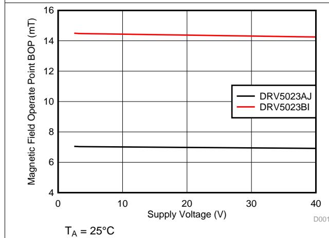
**Figure 3.  $B_{OP}$  vs  $V_{CC}$**
