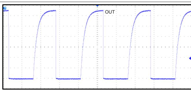
**Figure 22. 10-kHz Switching Magnetic Field**
