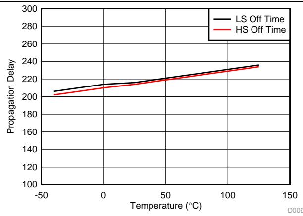
Figure 5. Propagation Delay Off Time vs Temperature
