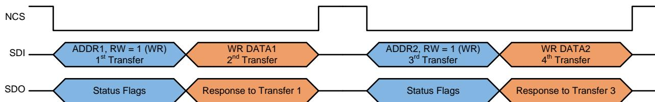
**Figure 13. Write Access Followed by Write Access**
