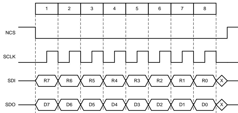
NOTE: SPI master (MCU) and SPI slave (DRV3205-Q1) sample received data on the !-falling!-rising SCLK edge and transmit on the !-rising!-falling SCLK edge.
