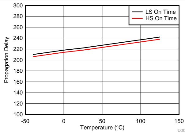
Figure 4. Propagation Delay On Time vs Temperature
