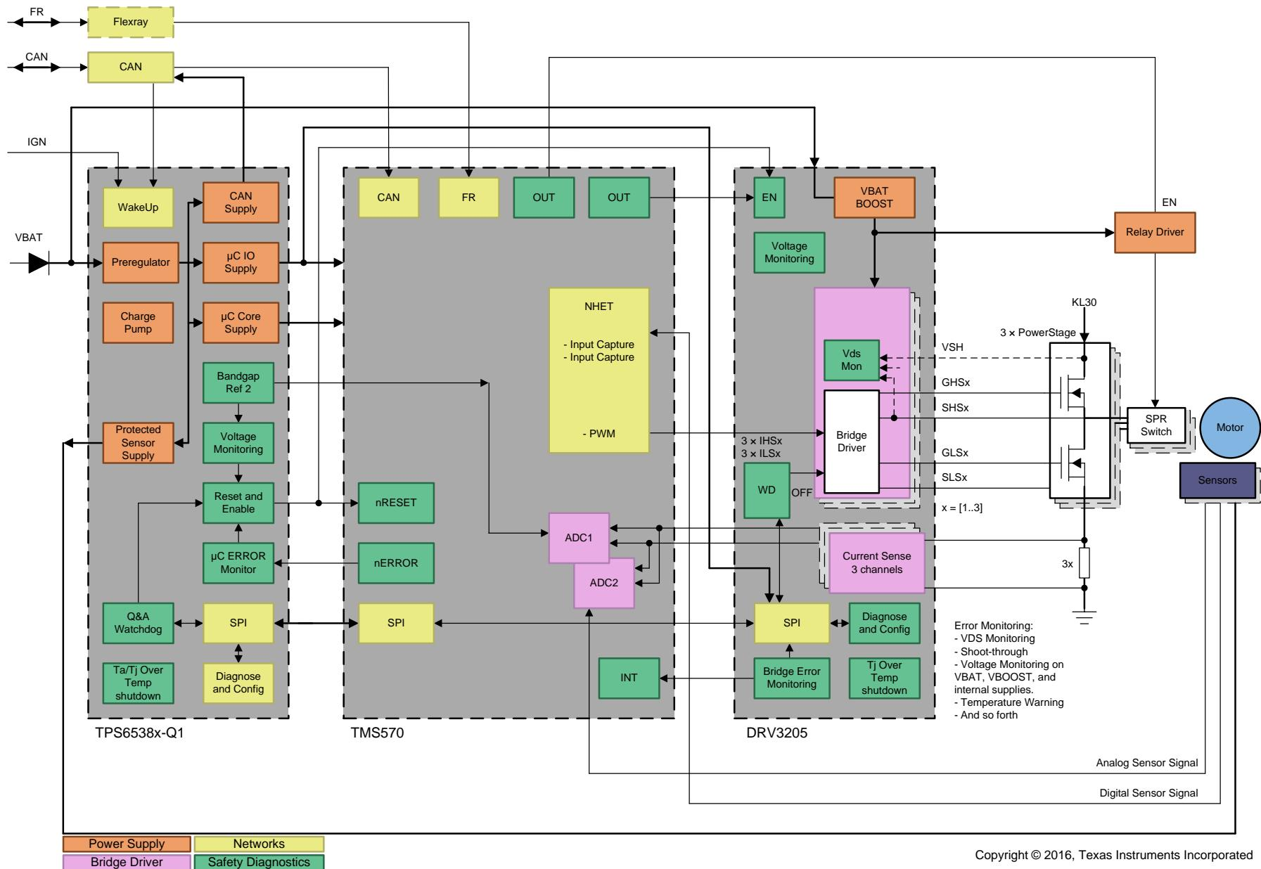
**Figure 18. Typical System – Electrical Power Steering Example**
