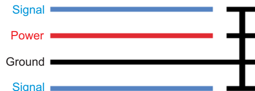
Figure 8-13. Guard Ring Routing
