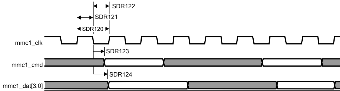
图 7-67. MMC/SD/SDIO in - High Speed SDR12 - Transmitter Mode
