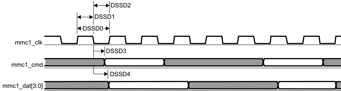
图 7-63. MMC/SD/SDIO in - Default Speed - Transmitter Mode
