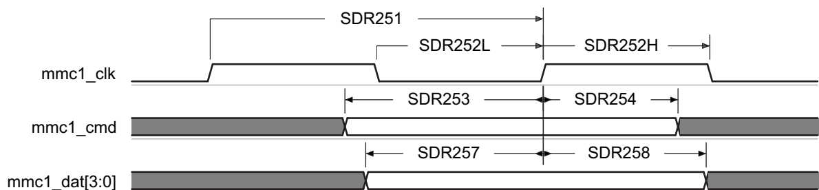
图 7-68. MMC/SD/SDIO in - High Speed SDR25 - Receiver Mode
