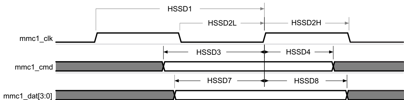
图 7-64. MMC/SD/SDIO in - High Speed - Receiver Mode
