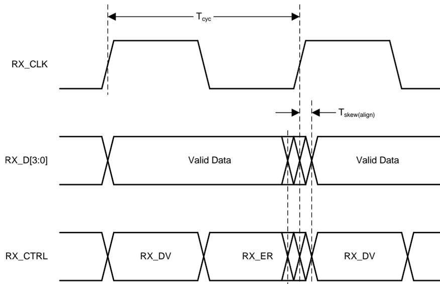
**Figure 7. RGMII Receive Timing (Internal Delay Disabled)**
