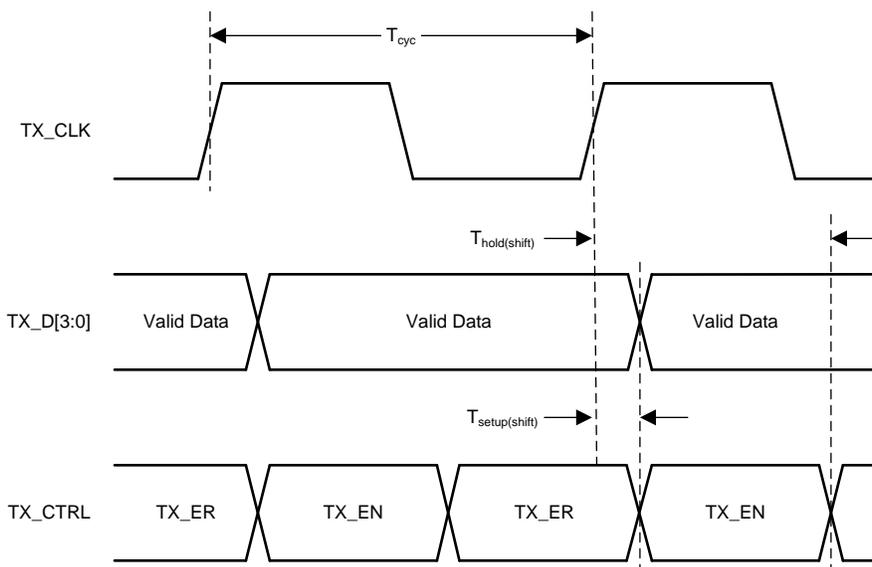
**图 4. RGMII Transmit Timing (Internal Delay Enabled)**
