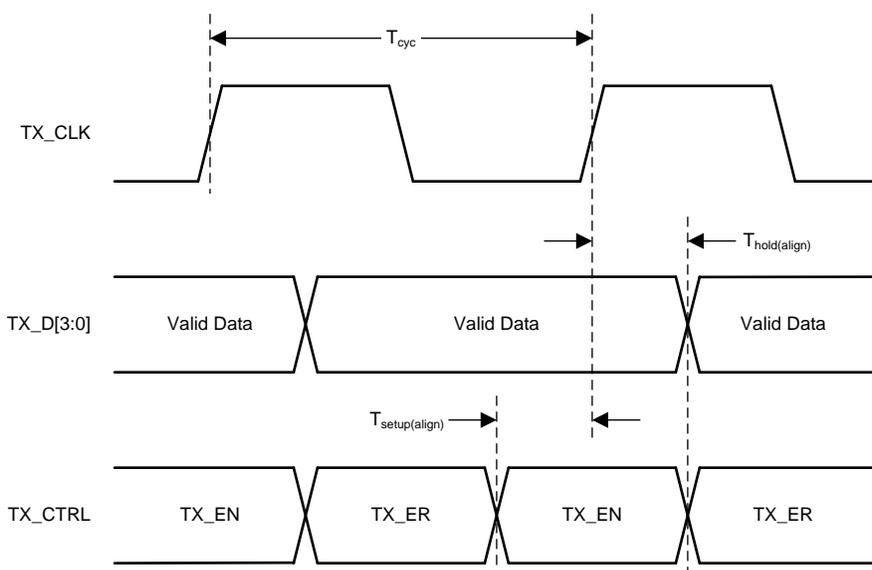
**图 5. RGMII Transmit Timing (Internal Delay Disabled)**
