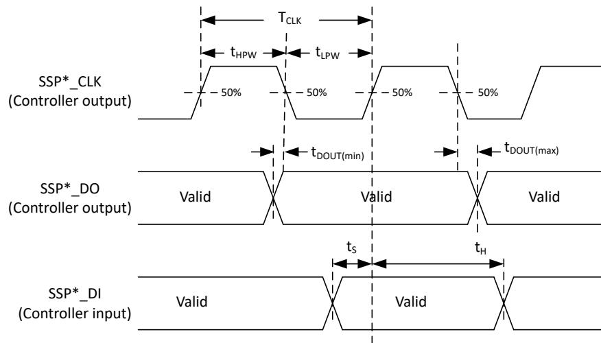
**Figure 5-13. Timing Diagram for SSP Target Mode (Modes 0/3)**
