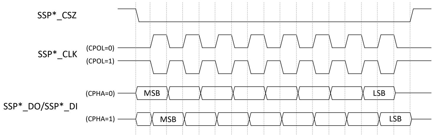
**Figure 5-11. Timing Diagram for SPI Clocking Modes**
