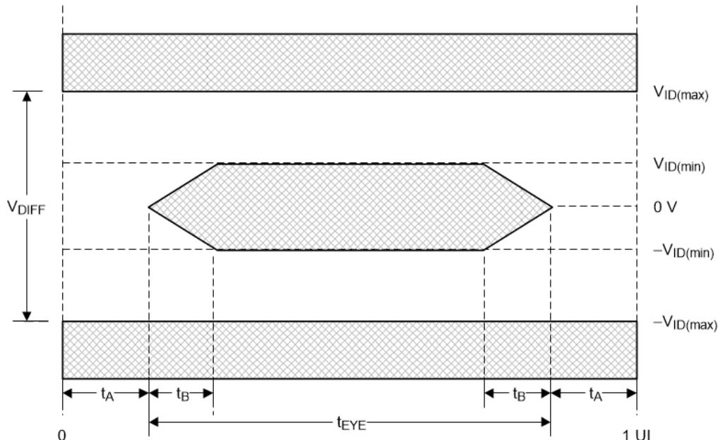
**Figure 5-8. V-by-One Timing**
