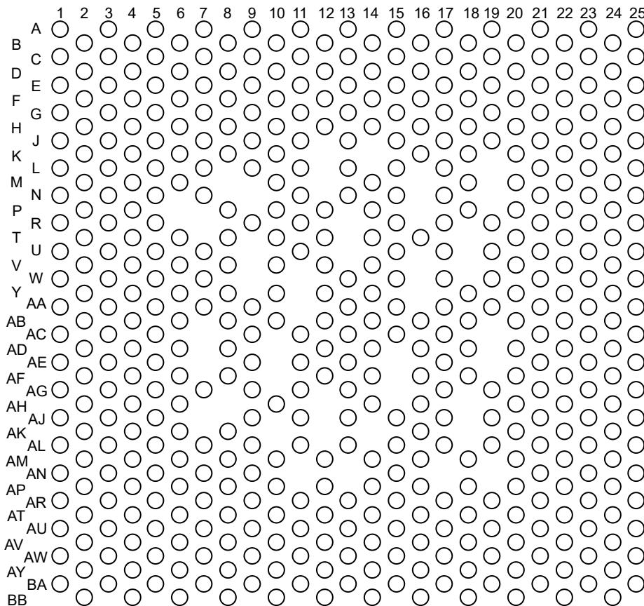
**Figure 4-1. AMD Package 484-Pin FCCSP Top View**
