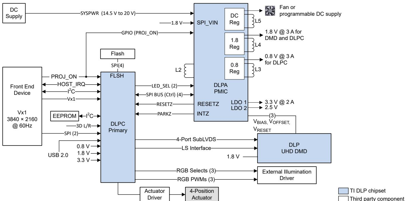
**Figure 6-1. LED Functional Block Diagram**
