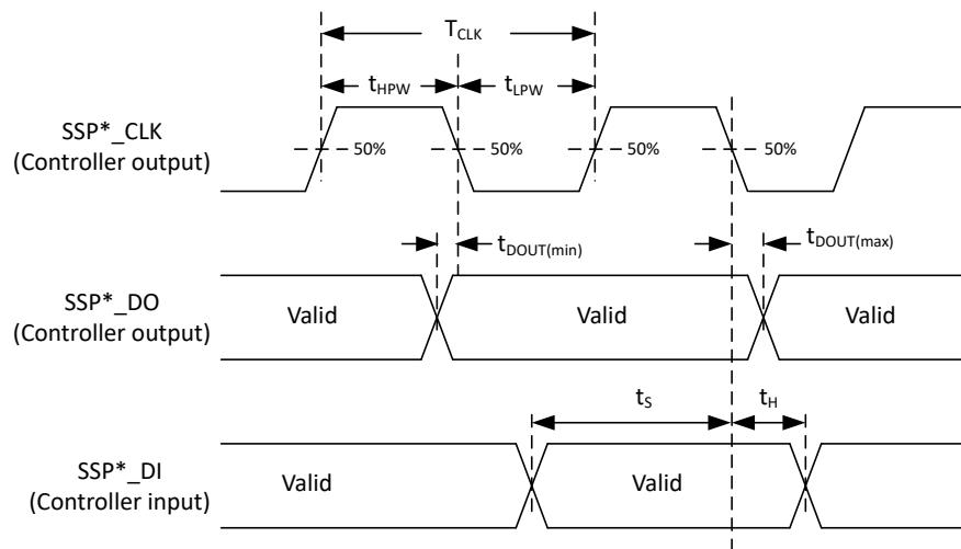
**Figure 5-12. Timing Diagram for SSP Host Mode (Modes 0/3)**
