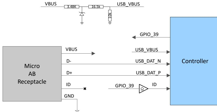
**Figure 5-5. USB Example for the DLPC8445 Controller**
