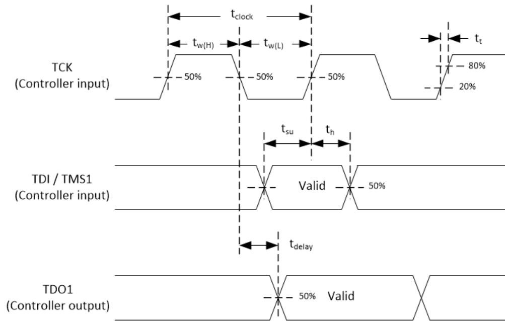
**Figure 5-14. Timing Diagram for JTAG Boundary Scan**
