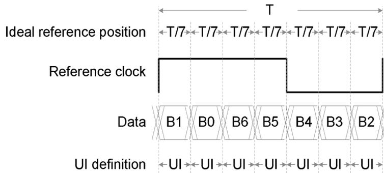
Figure 9. (LVDS) Clock – Data Skew Definition
