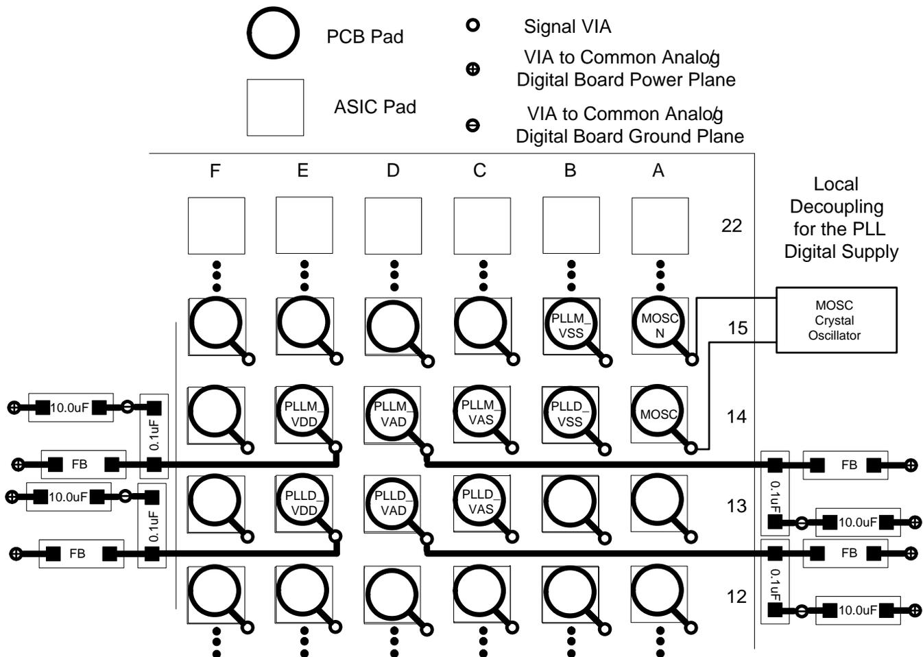
Figure 18. PLL Filter Layout
