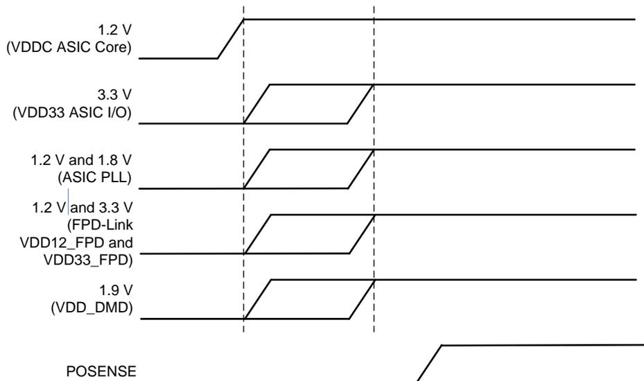
**Figure 16. System Power-Up Sequence**
