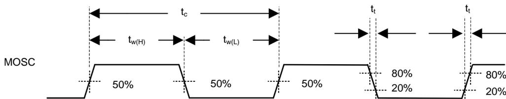
Figure 1. System Oscillators
