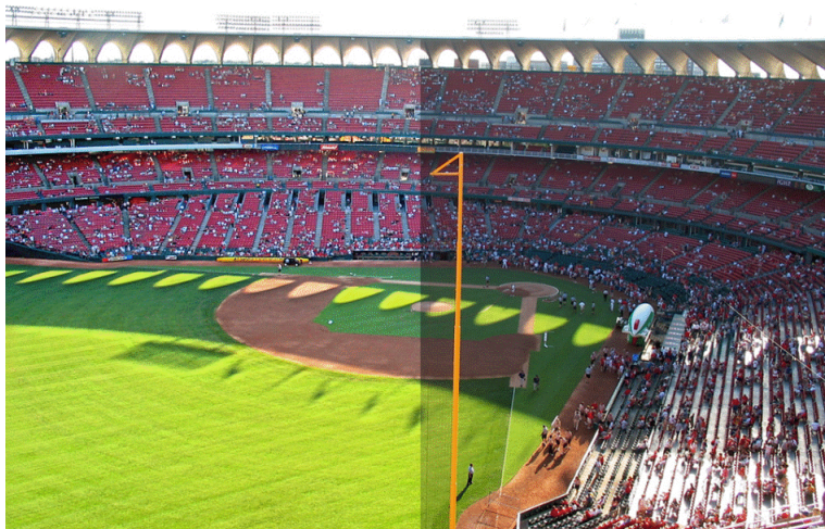
Figure 7-13. LABB enabled (left side) and LABB disabled (right side)
