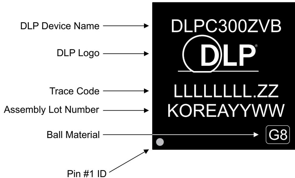
**Figure 25. Device Marking**
