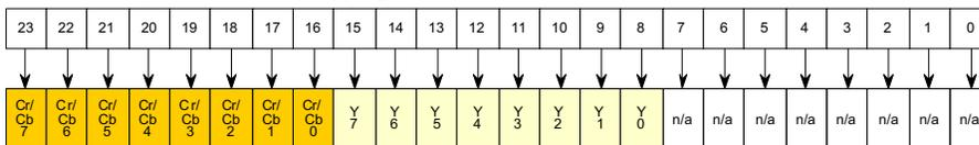
PDATA(23:0) of the Input Pixel data bus
