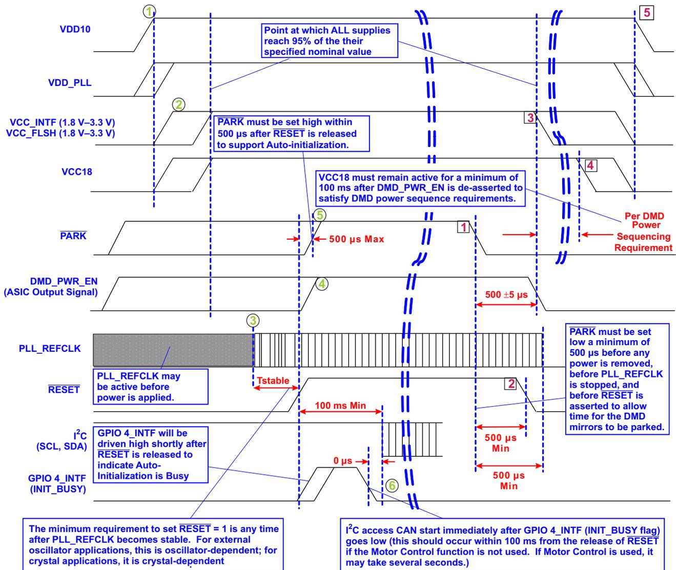
Figure 17. Power-Up/Down Timing
