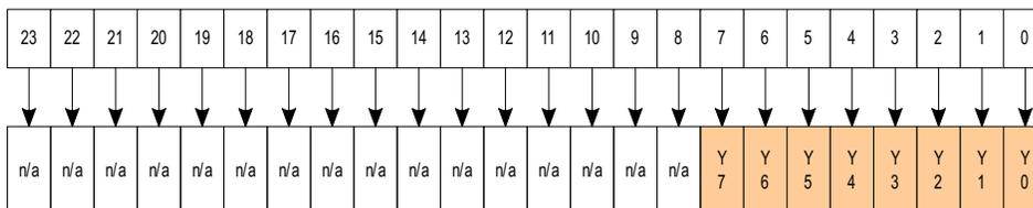
PDATA(7:0) of the Input Pixel data bus
