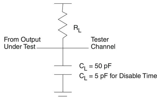
**Figure 7-4. Test Load Circuit for AC Timing Measurements**
