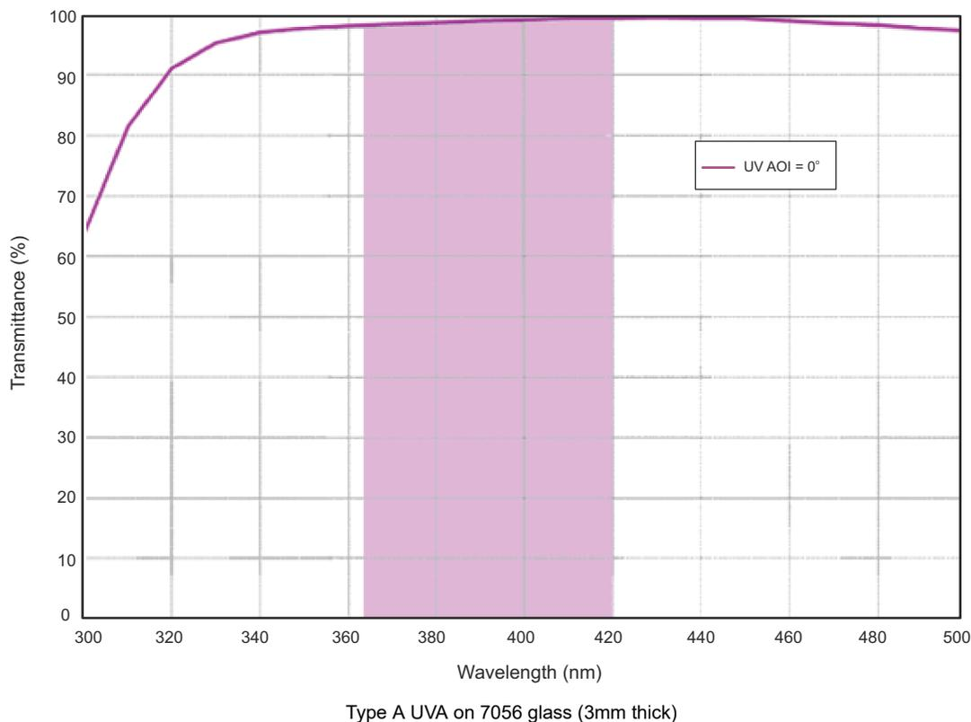
図 8-3. Corning 7056 UV Window Transmittance (Maximum Transmission Region)
