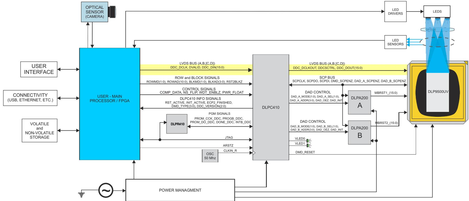
図 8-2. DLPC410 and DLP9500UV Embedded Example Block Diagram
