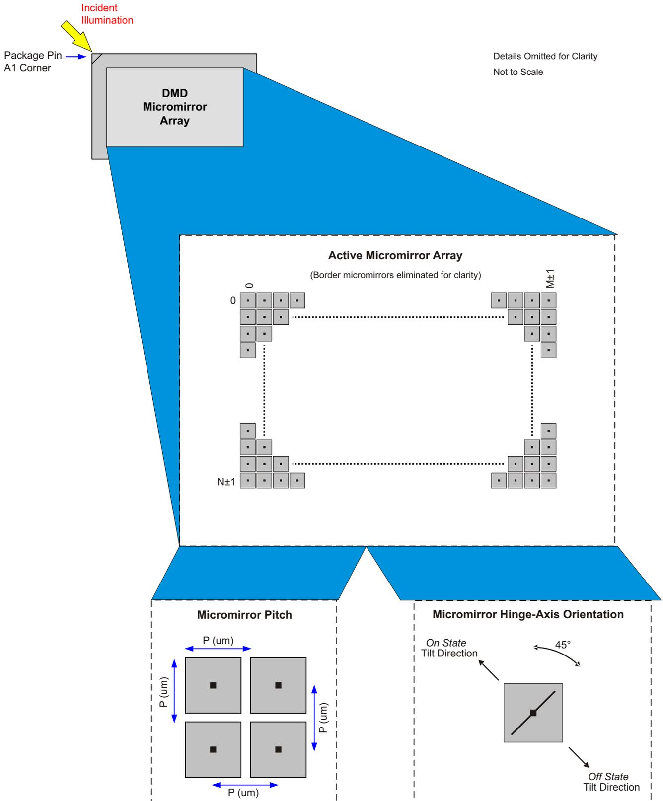
図 7-5. DMD Micromirror Array, Pitch, and Hinge-Axis Orientation
