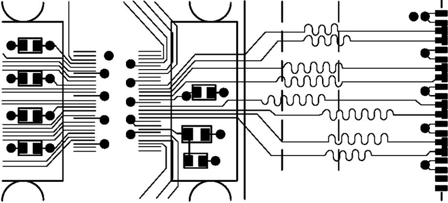
図 8-4. Mitering LVDS Traces to Match Lengths
