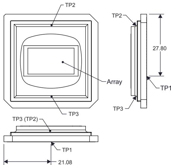
**Figure 7-11. Thermal Test Point Location**
