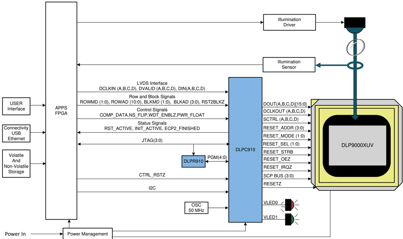
Figure 20. DLP9000XUV DMD - Typical Application Schematic
